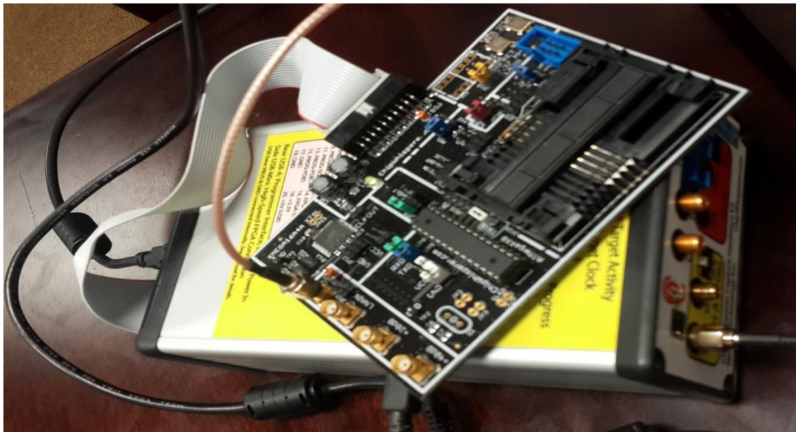
Figure 3.2: The complete system, including the FPGA board from Figure 3.1 which is mounted in an enclosed case, and the example capture board from Figure 3.3.
