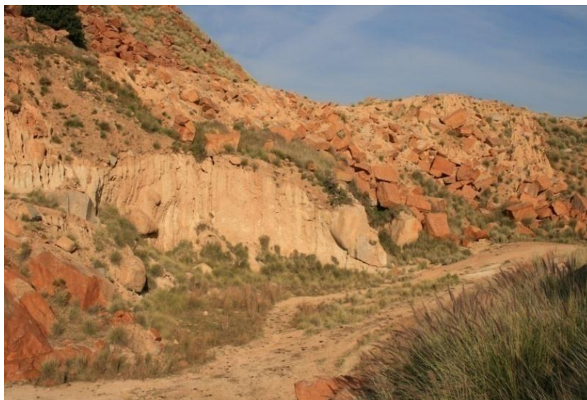
Figure 76. Granite blocks at Leeukop Quarry (GQ3 Kopjeskraal 517 IQ) are stained with an iron oxide in an attempt to blend the freshly exposed granite with the natural environment.
