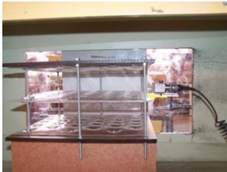
Figure 22: Model for aspect ratio of 2 with mounted accelerometer
