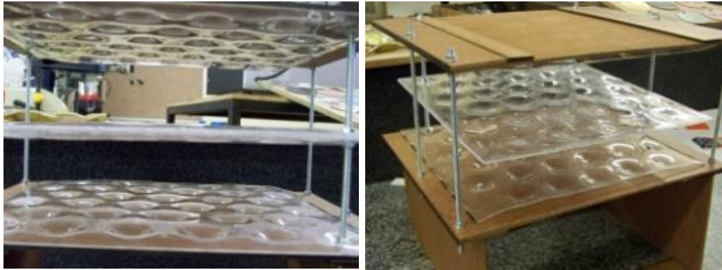
Figure 12: Flow model assembly, dimple plate between two formed Perspex sheets
