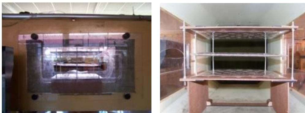
Figure 14 : The flow-model mounted in the wind tunnel
