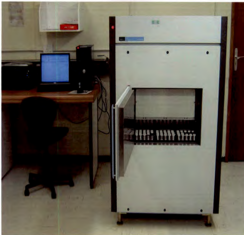
Figure 4.4. The Wallac Quantulus 1220™ (PerkinElmer Life and Analytical Sciences) frontal view with open lid, showing the auto sampler trays
