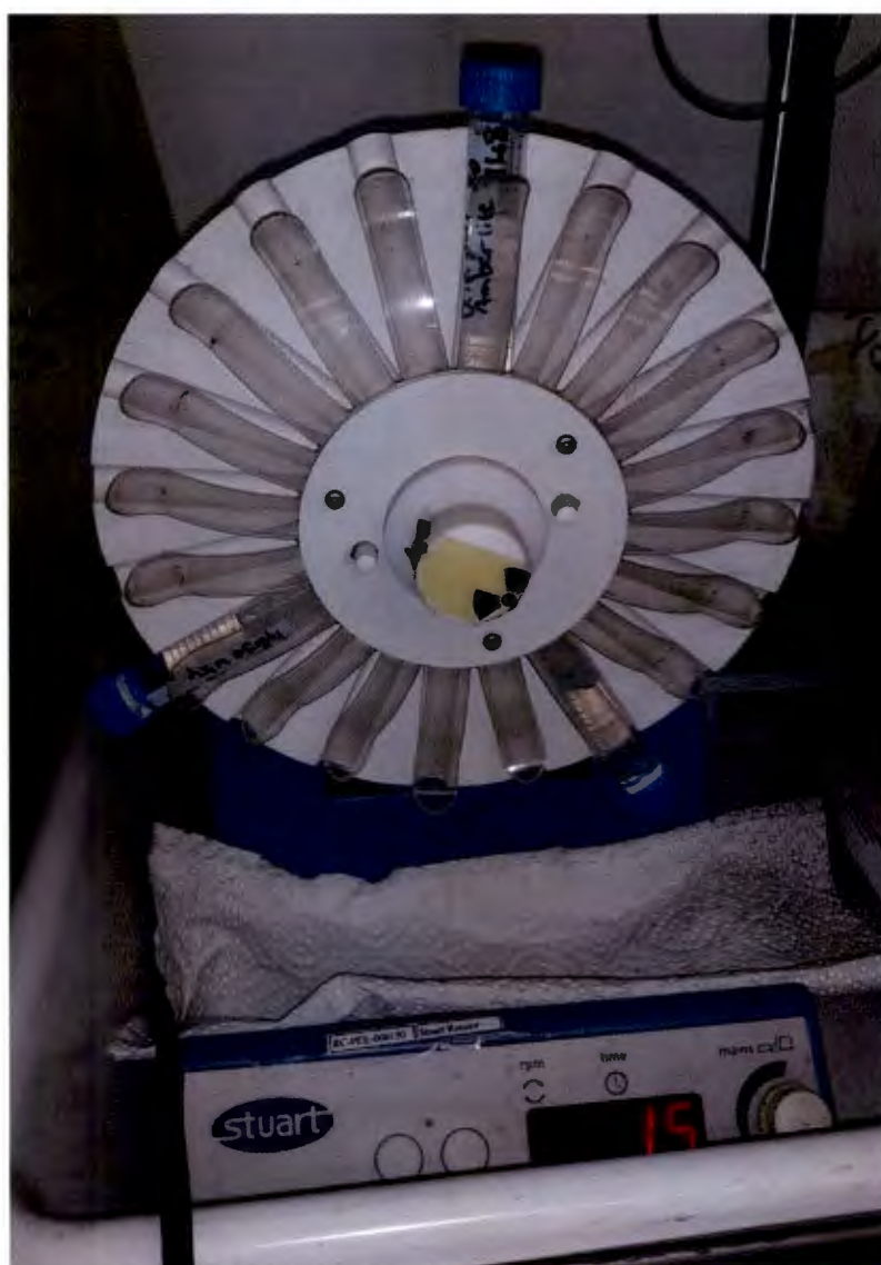
Figure 3.6: Uranium solution contacted with three resins to determine the distribution efficiency of each.
