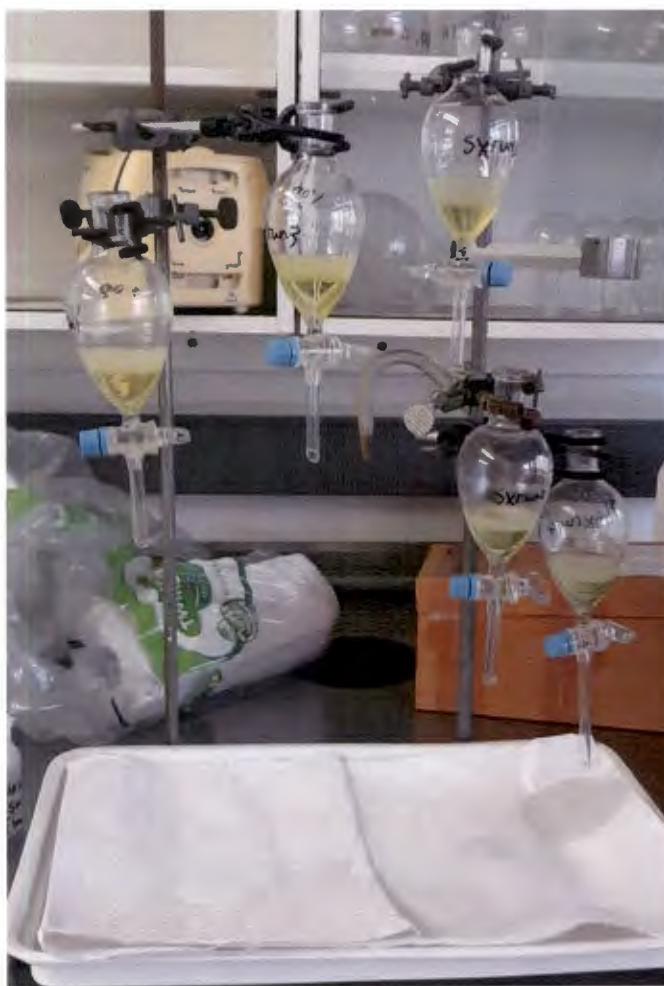
Figure 3.4: Organic phase and aqueous (uranium solution) phase in separatory funnels settling after being contacted with one another.
