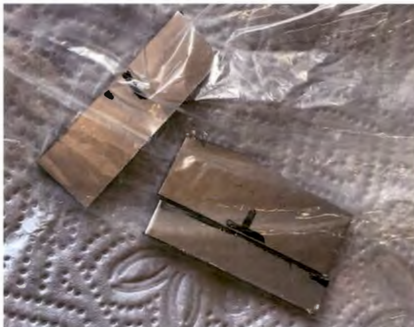
Figure 3.3: ¼ of TP that has been sheared further to smaller pieces.
