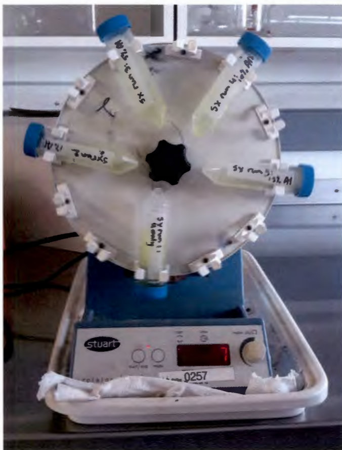
Figure 3.5: Process of stripping uranium from organic phase using 0.5 M (NH 4 ) 2 CO 3 .
