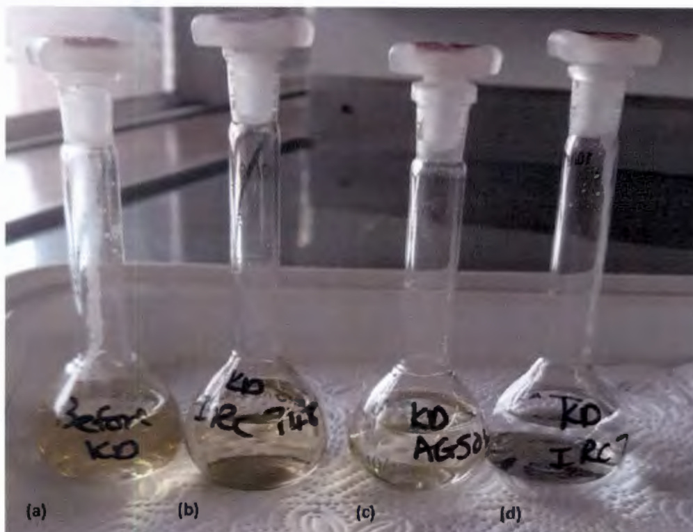
Figure 4.20: (a) Solution before using resin, (b) solution after using Amberlite IRC748, (c) solution after using AG50W-X4, and (d) solution after using Amberlite IRC747.
