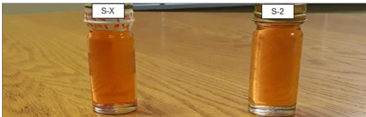
Figure 4.12: Stretford™ circulation solutions appearance with and without impurities at \text{V}^{5+} of 0.029 \text{ mol.dm}^{-3}
