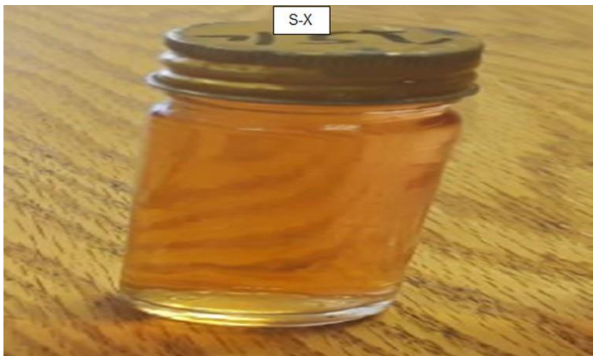
Figure 4.3: Synthetic Stretford™ aqueous solution without impurities ( \text{Na}_2\text{SO}_4 and \text{NaSCN} )
