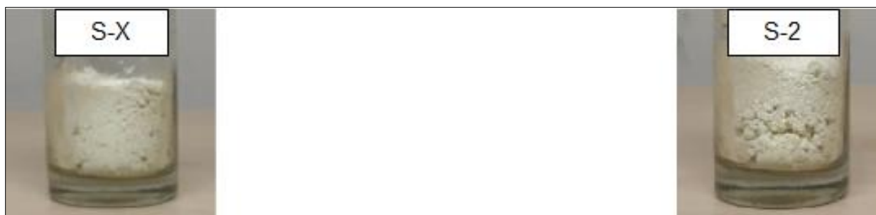
Figure 4.13: Elemental sulphur produced concentrations with and without impurities
