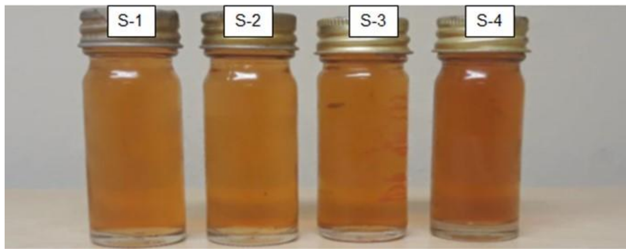
Figure 4.1: Stretford™ aqueous solutions physical appearance at different V^{5+} concentrations
