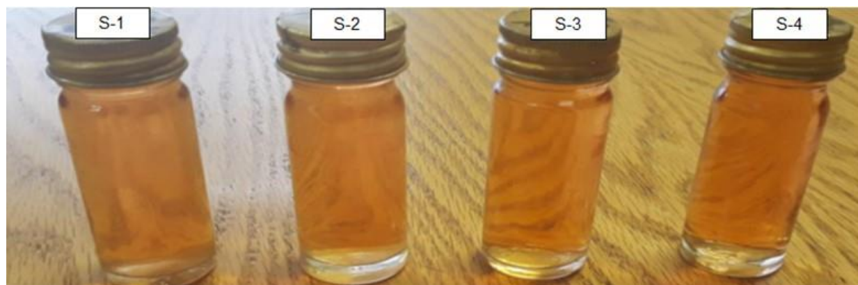
Figure 4.5: Stretford TM circulation solutions appearance at different V^{5+} concentrations
