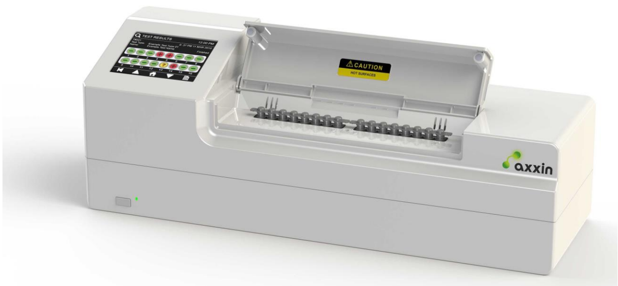
Figure 3.2: The Axxin T16 isothermal instrument with 16 positions for loading tubes with samples and a touch result screen for real-time monitoring
