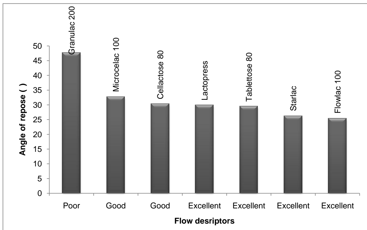
Figure 3.4: Angle of repose of various lactose-based filler/binders.
