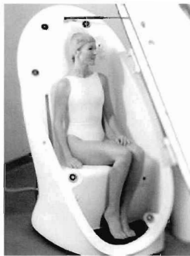
Figure 2.1 The Bod Pod air displacement plethysmograph adapted from Life Measurement, Inc. (2007)
