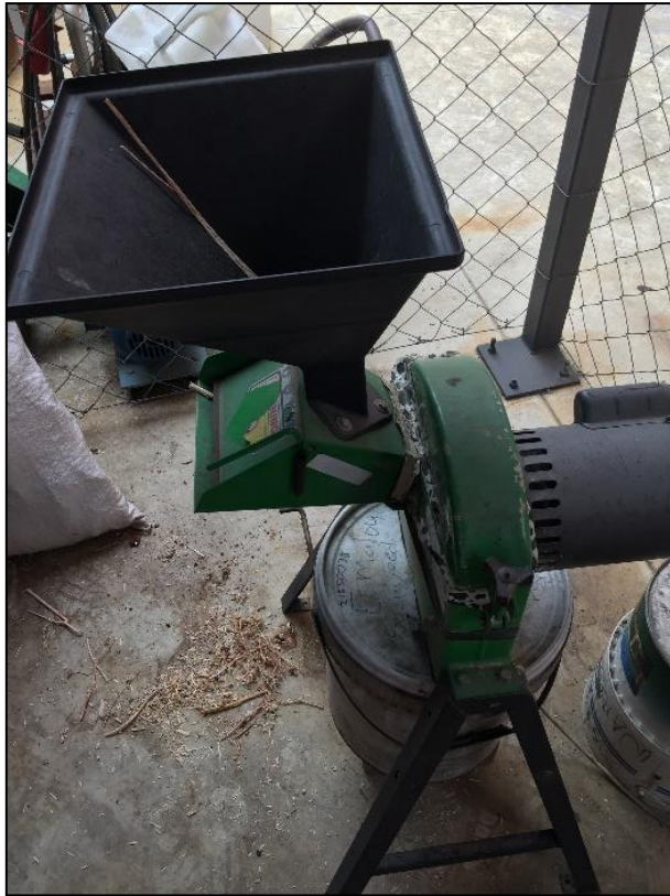
Figure 3-2: Hammer mill used to reduce particle size (left) and grounded quinoa lignocellulose (right)
