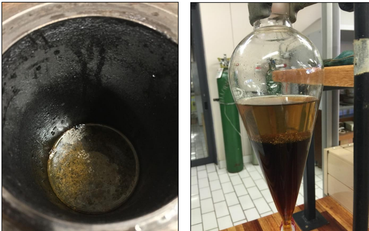
Figure 3-5: Autoclave content after liquefaction (left) and separation of water and bio-oil using a separatory funnel (right)
