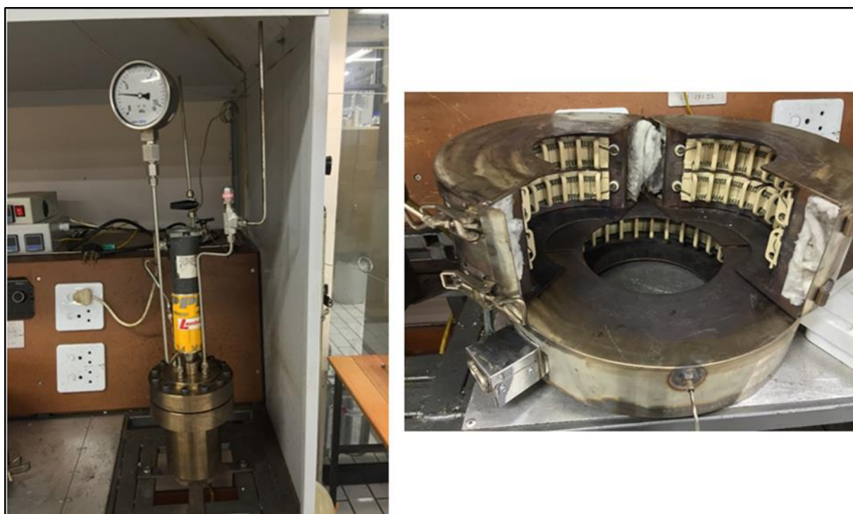
Figure 3-4: Autoclave with magnetic stirrer (left), Removable heating jacket (Right)
