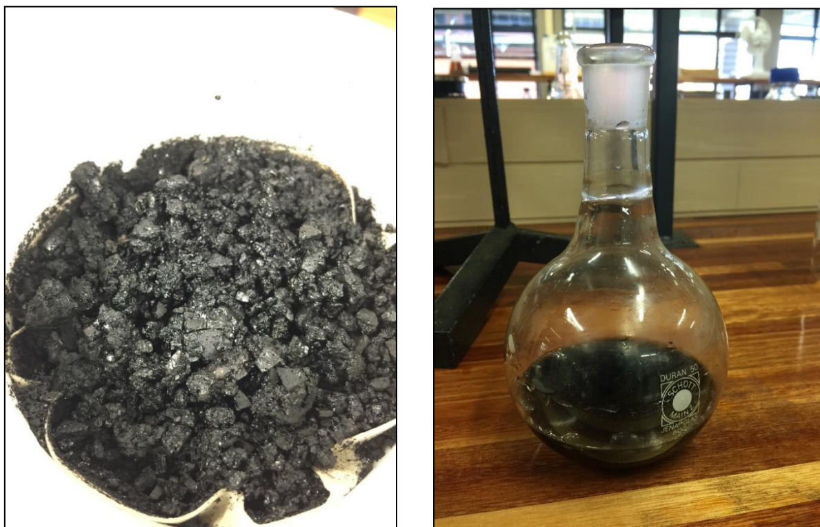
Figure 3-6: Separated biochar (left) and bio-oil (right) before drying
