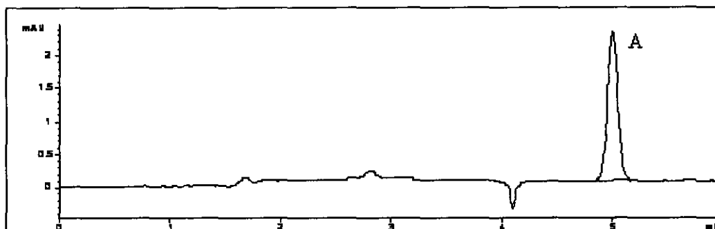
Figure 3-8: The 5-fluorouracil peak (A) was obtained with a 0,1 µg/ml standard solution of 5-FU in HPLC grade water. The AUC was 28,86 mAU and the retention time was 4,99 min.
