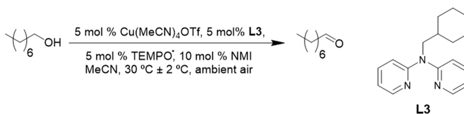
Scheme 10. A (L3)Cu I /TEMPO·/NMI catalyst system the aerobic oxidation of 1-octanol to 1-octanal under synthetically relevant reaction conditions [10]. Reproduced with permission from Swarts and co-workers. Copyright Royal Society of Chemistry, 2017. Successful oxidation was possible for a variety of primary alcohols (65 to 98%). The selectivity of the catalyst system was not evaluated.
