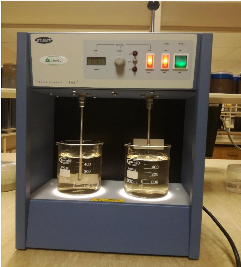
Figure 13: SW5 flocculator with variable mixing speeds.
