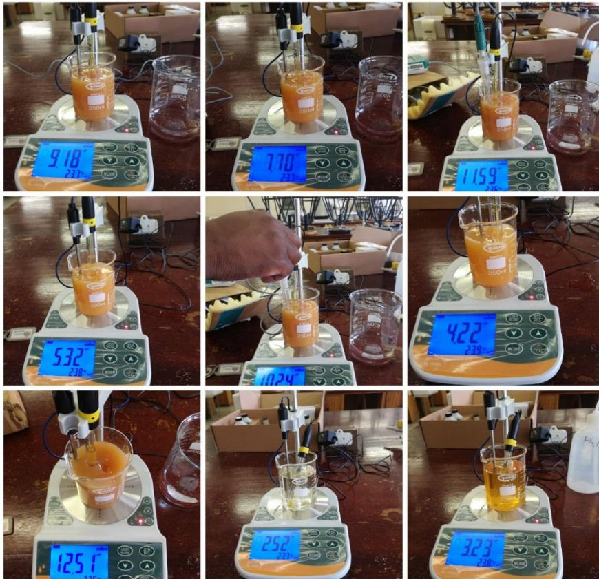
Figure 22: Picture collage showing steps in the evaluation of the 2.5 M NaOH solution for pH adjustment purposes.
