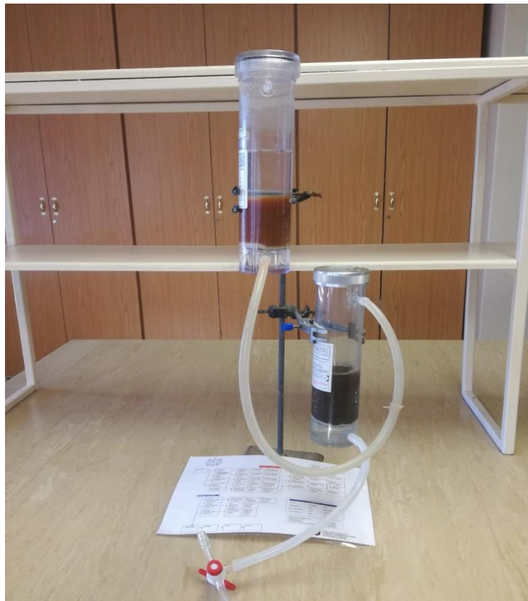
Figure 15: Experimental setup for ion exchange treatment.
