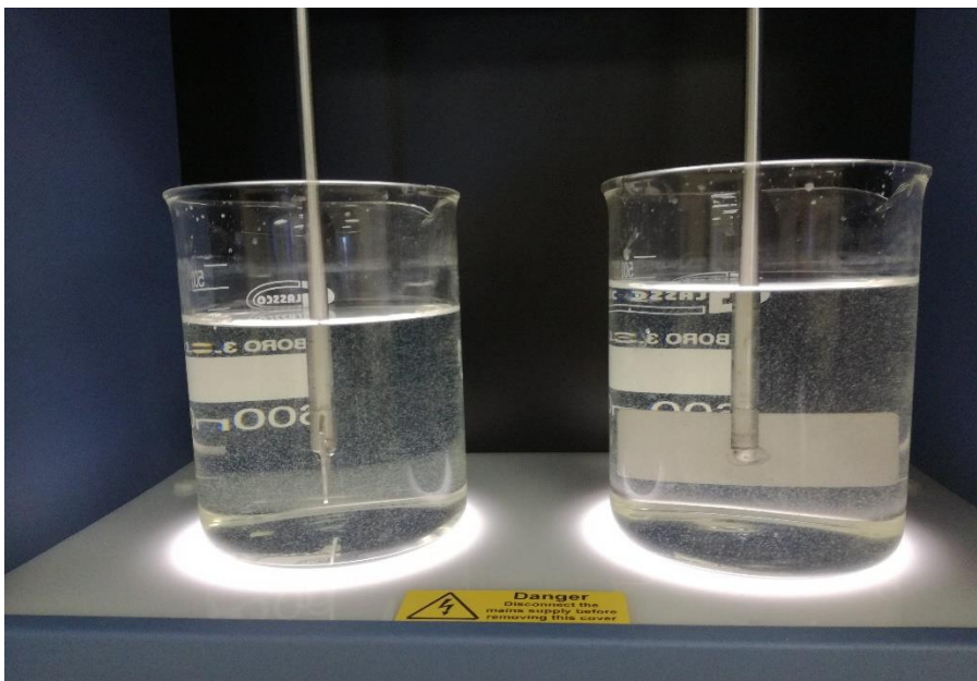
Figure 14: Macro-flocs forming during the slow mixing stage of coagulation/flocculation.
