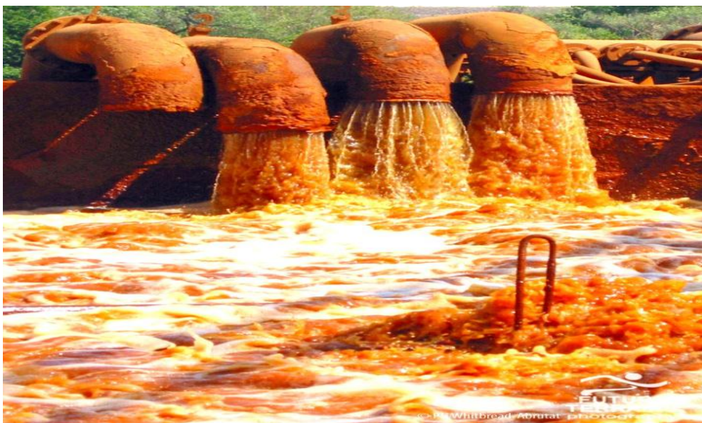
Figure S10: AMD pumped from underground
