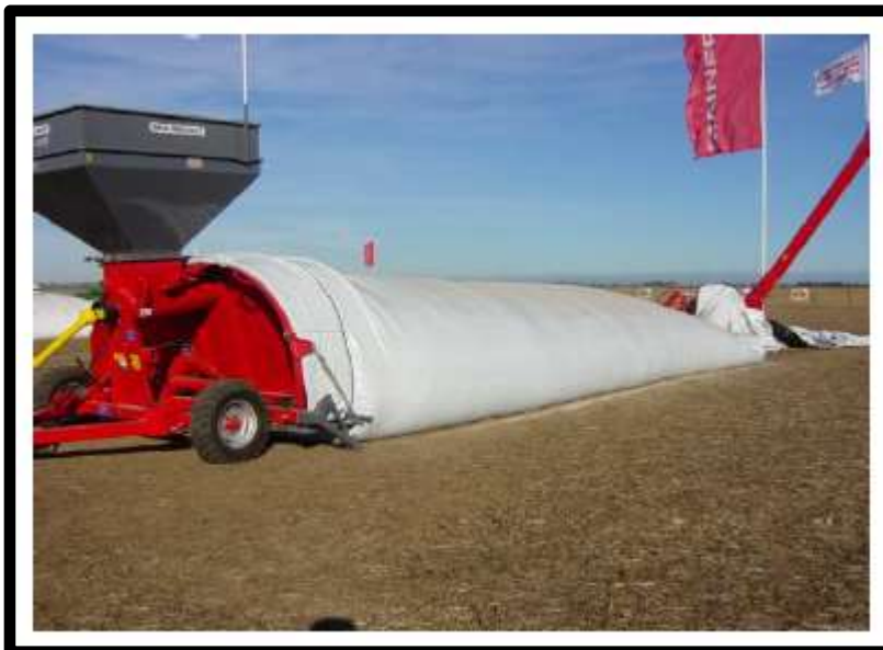
Figure 2.8 – Silo bag loading system.
