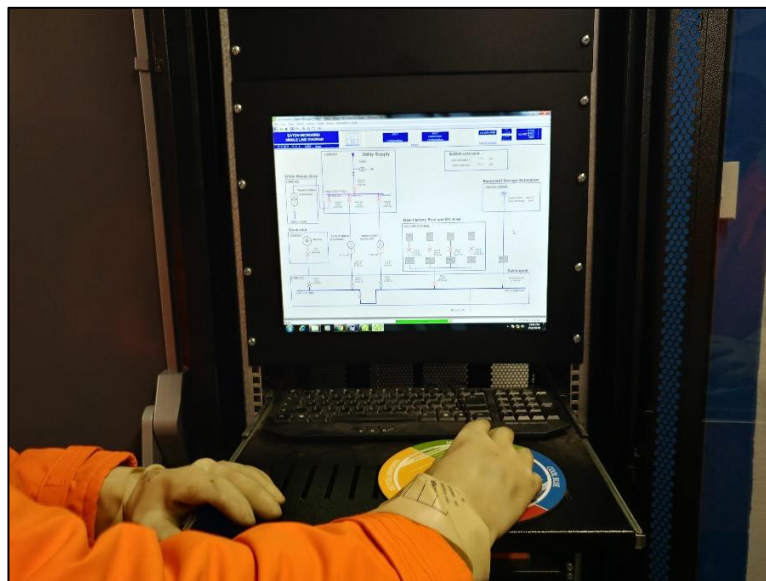
Figure 2: HMI for Controlling Storage System
