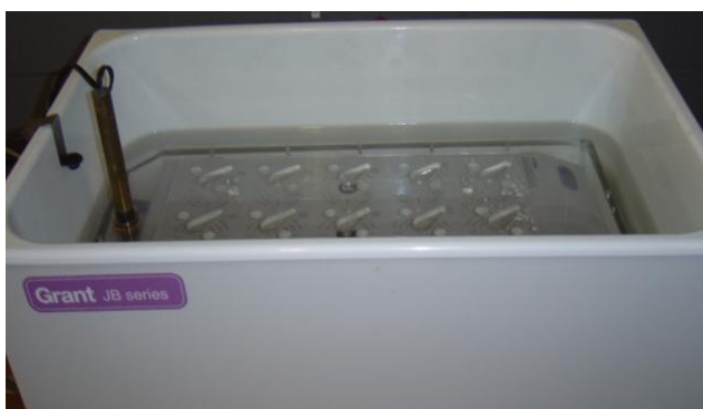
Figure D.2: Grant water bath fitted with a Variomag magnetic stirrer plate and Franz cell stand
