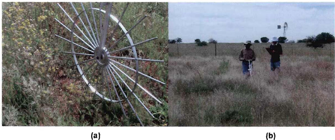
Figure 3.8 The wheel-point apparatus used in this study and how the surveys were carried out at the trial site.
