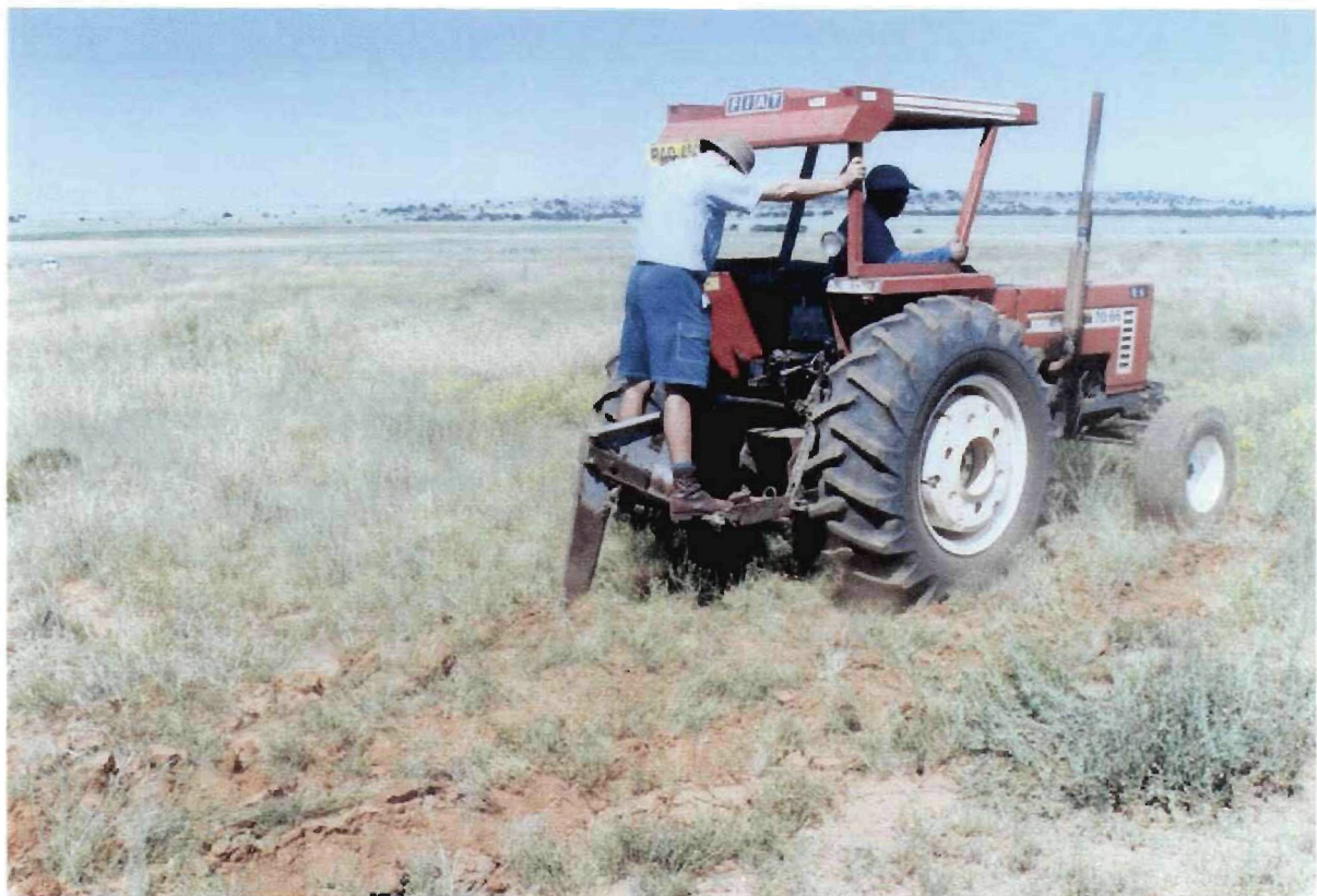
Figure 3.1 The rip action applied in this study, by means of a one tine ripper.
