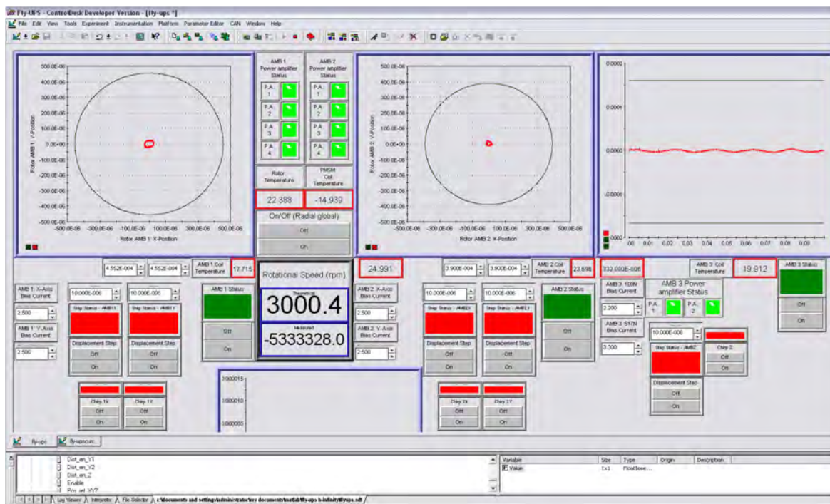
Figure 5.2-3: Fly-UPS rotor positions on ControlDesk® GUI
