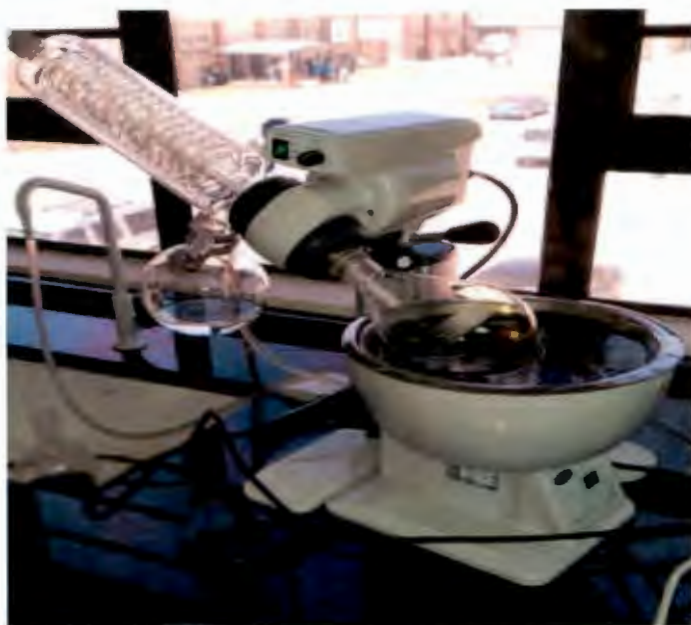
Figure 4: Rotary evaporator used to remove organic solvents
