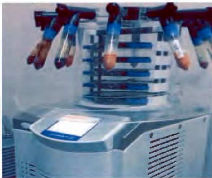
Figure 5: Lyophilizer (Freeze Dryer) used to remove water from crude extract.
