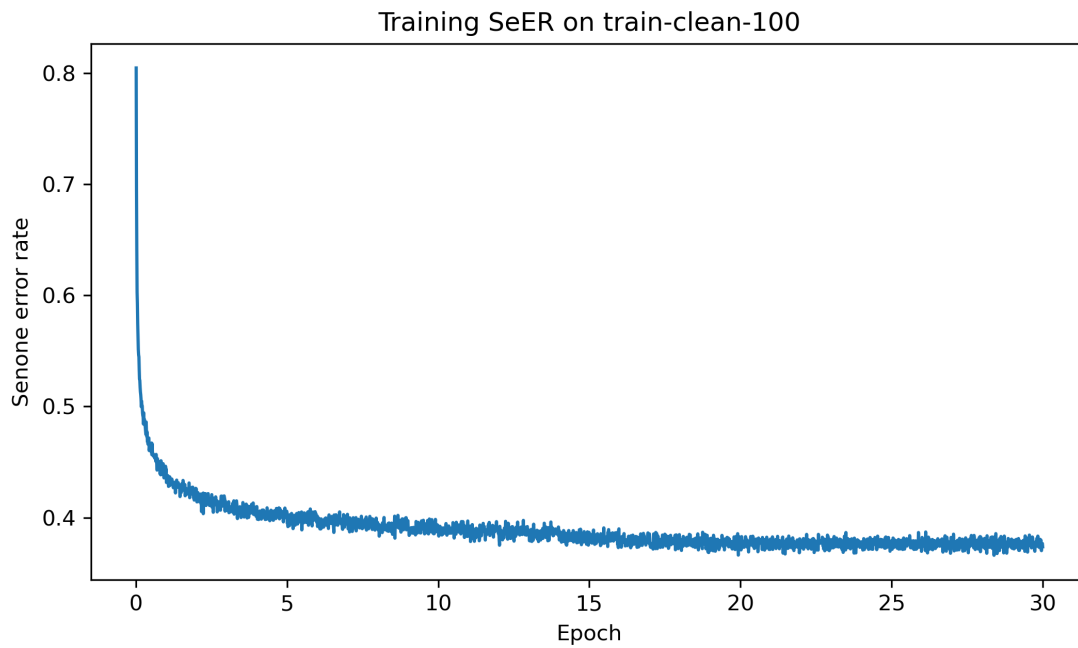
Figure 4.1: SeER measured on train-clean-100 subset of the LibriSpeech corpus using the MLP baseline acoustic model.
