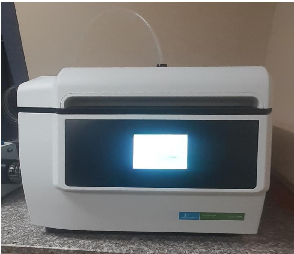
Figure 3. 6: The titan MPS™ microwave digester used in sample digestion.
