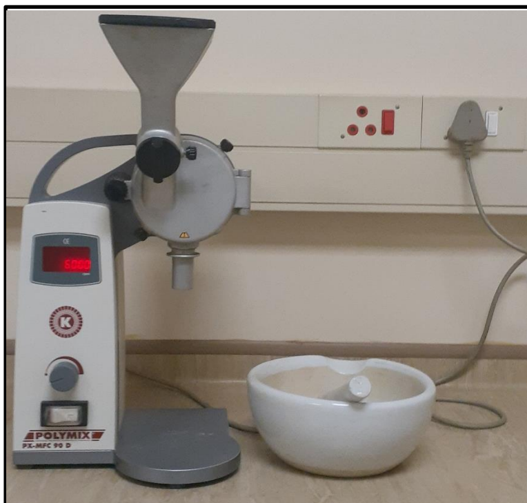
Figure 3. 5: Milling and crushing instrument used in sample preparation.
