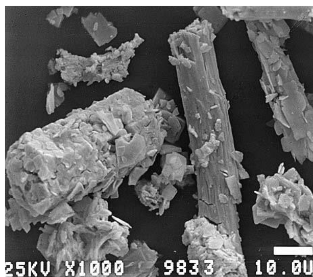
Figure 3. 11: SEM picture of PuO 2 platelets from a sample seized in 1994 at Munich airport, Germany (Ho, 2015).
