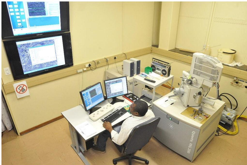
Figure 3. 9: The FEI Quanta FEG 250 Electron microscope at North-West University ( http://natural-sciences.nwu.ac.za/laboratory-electron-microscopy/home-0 : 01 February 2022).
