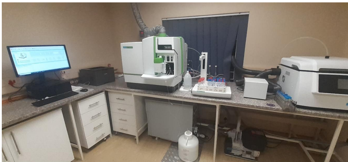
Figure 3. 8: The ICP-MS NexION 2000C instrument at CARST for multi-elemental analysis.
