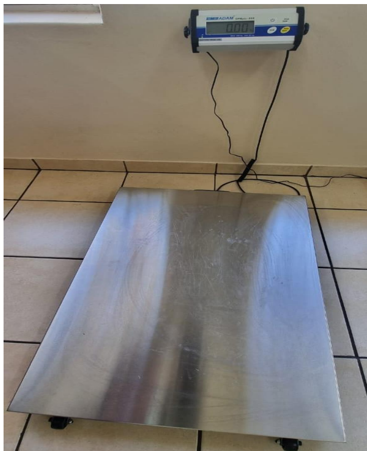
Figure 3. 4: The Adam TCS150 platform scale used for weighing the samples.
