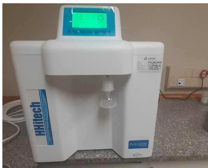
Figure 3. 7: Ultrapure HHitech laboratory water purification system.
