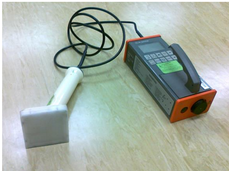
Figure 3. 3: Electra-GM radiation instrument used for contamination monitoring.
