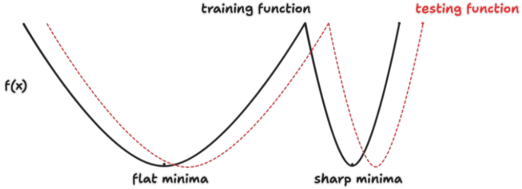
Figure 2.3: A sketch of valleys with flat minima vs. sharp minima. This illustrates the high sensitivity of a training function to perturbations, which negatively affects generalization. Regions with flat minima are less complex and require low precision weights, making them likely to generalize better. Adapted from [33].
