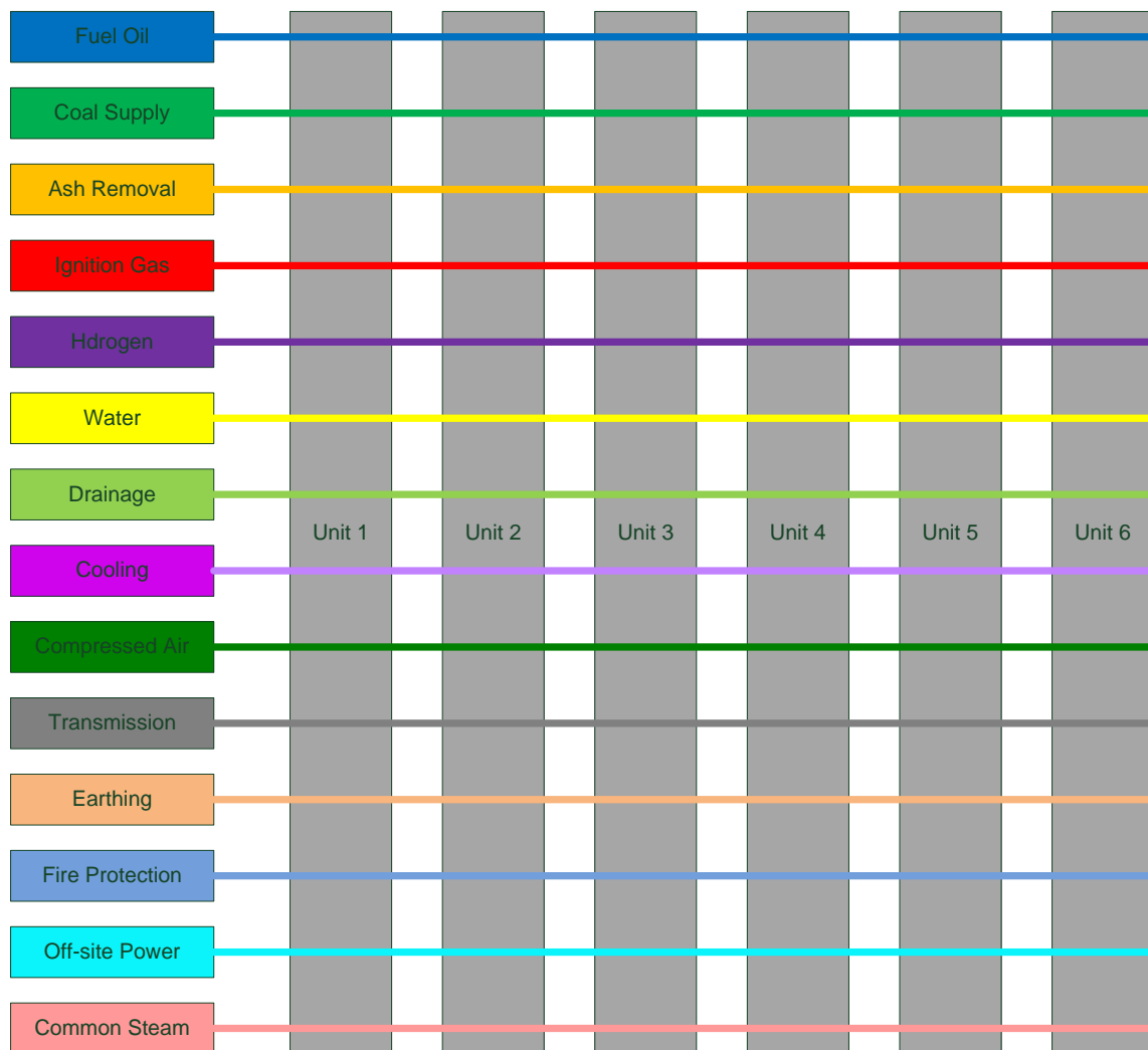
Figure 52: Power station systems supporting multiple generating units
