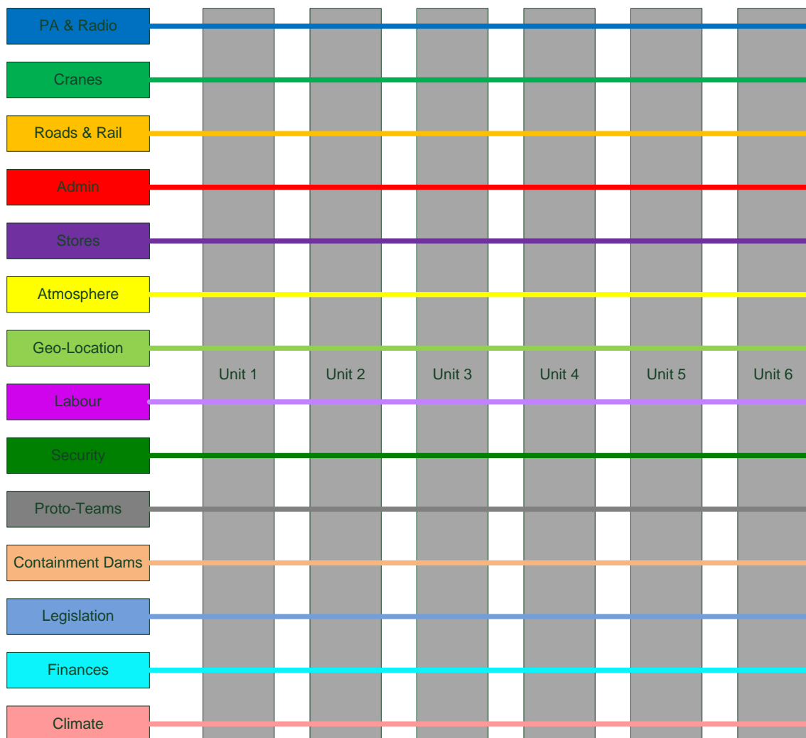
Figure 53: Power station non-production systems supporting multiple generating units
