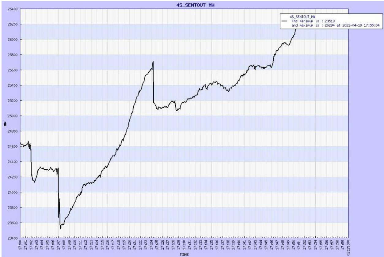
Figure 117: Total power system power send out for the Lethabo event of 19 April 2022
