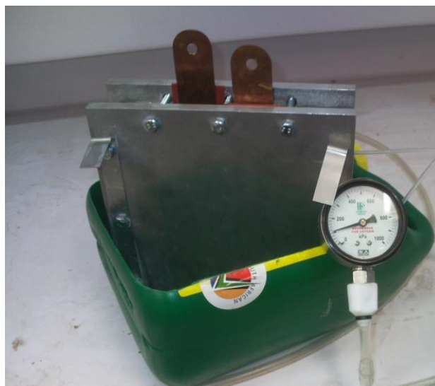
Figure 40: Gas leakage test set-up with a pressurized oxygen supply (not shown) coupled to the electrolyzer
