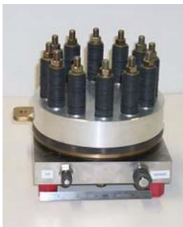
Figure 6: PEM electrolyzer stack assembly with 3 internal MEA's [8]
