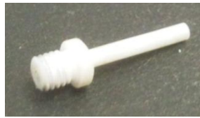
Figure 31: M3 ISO threaded inlet and outlet components manufactured from PTFE
