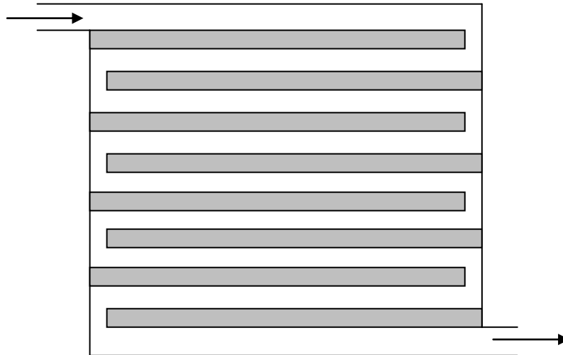
Figure 12: Serpentine flow field design modified after L. Xianguo et al. (2005)
