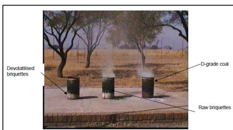
Figure 2.4: Combustion tests: Comparison of devolatilized binderless briquettes, raw binderless briquettes and D-grade sized coal (Mangena, 2004).
