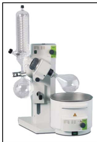
Figure 4.5: Rotary evaporation setup.
