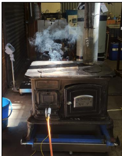
Figure 4.7: Union 7 coal stove investigated during combustion experiments.
