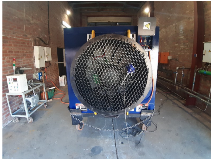
Figure 27: Axial fan fitted to the front of an ACU (Source: Author's own depiction)
