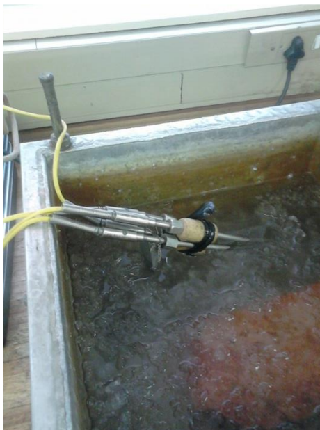
Figure 23: Calibration of thermocouples
