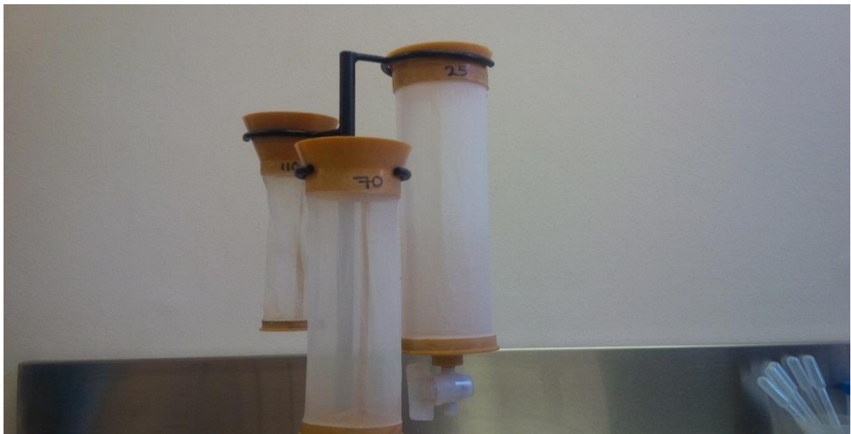
Plate 5.3: The sieves of 117, 70 and 25 \mu\text{m} used to recover nematode eggs from the sheep pellets
