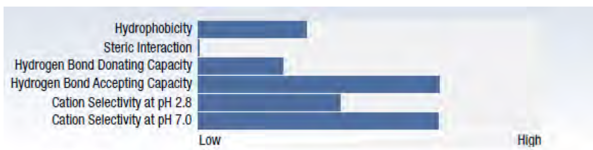
Figure 4.12: The selectivity profile of the Synergi Polar-RP column (Phenomenex, 2013, 2015).
