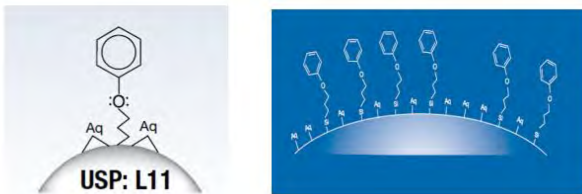
Figure 4.11: The chemical composition of the packing material inside the Synergi polar-RP column (Phenomenex, 2013, 2015).
