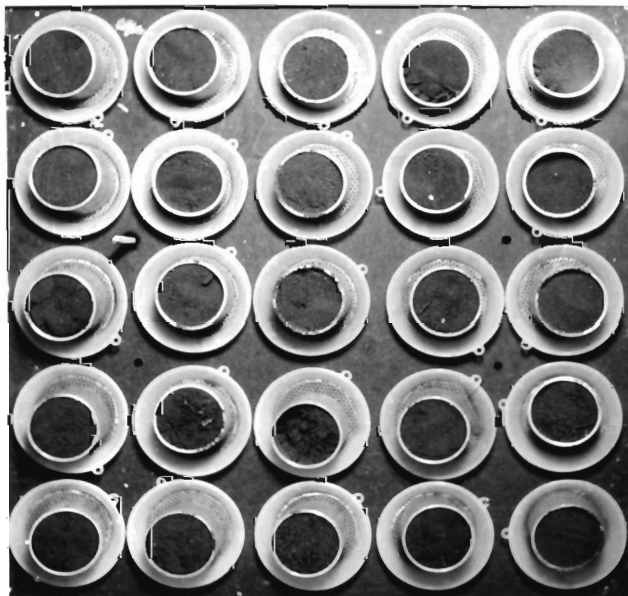
Plate 11 : Subsamples seen from above in funnel extraction unit.
