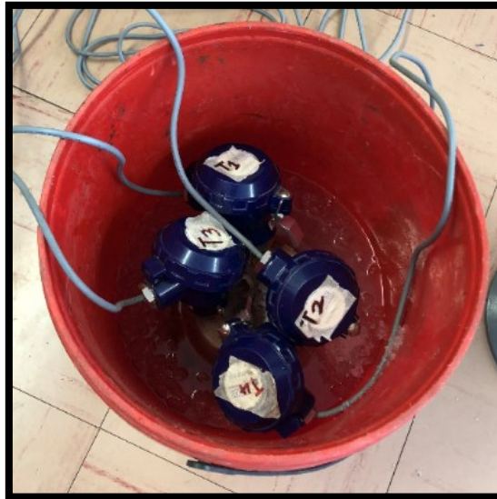
Figure 4-12: Four three-wire PT 100 sensors submerged in an ice bath.
