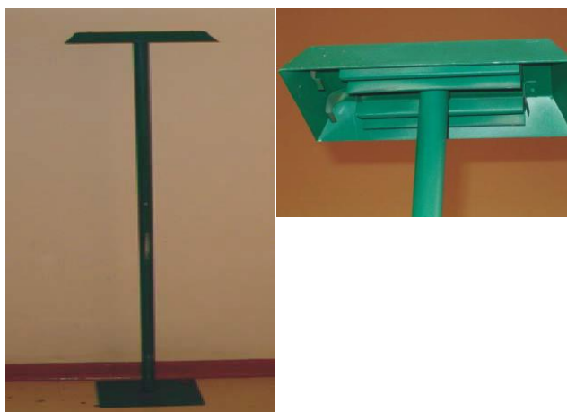
Figure 3.2: Aluminium stand (left) and the housing unit (right) wherein passive samplers were placed for exposure each month at the South African DEBITS sites (Martins et al. , 2007)
