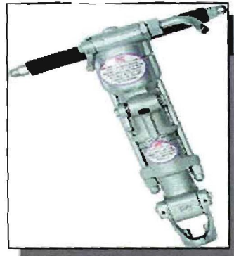
Figure 2-1 An example of a rock drill
