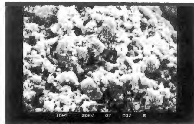
Micrograph 5.8 Surface of monolith wash-coated with commercial powder.
