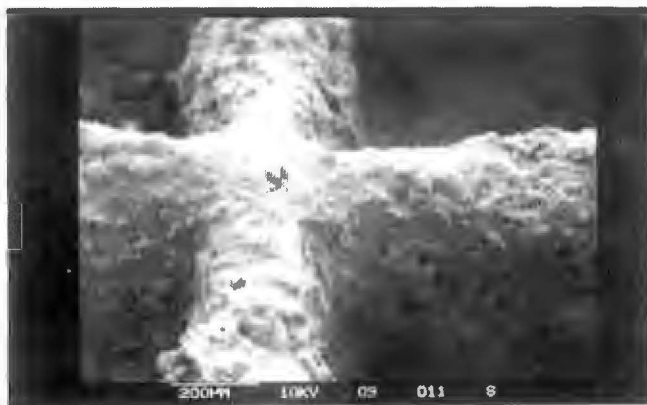
Micrograph 5.7 Monolith wash-coated with commercial powder milled for 12 h.
