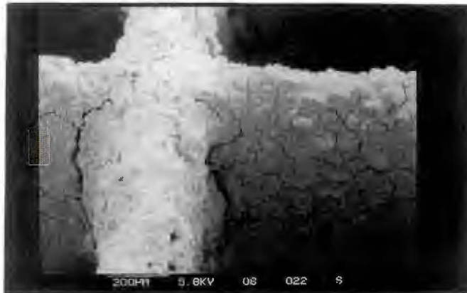
Micrograph 5.6 Typical poor coating with commercial alumina powder.
