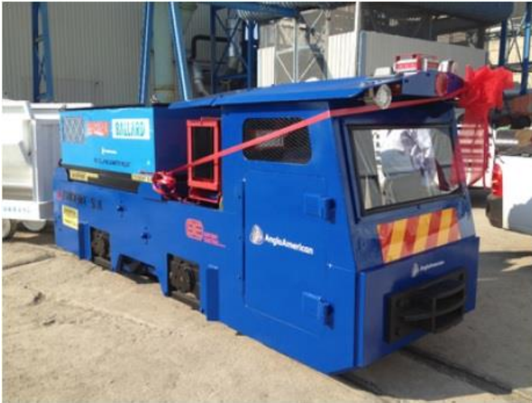
Figure 2-2: Anglo American locomotive prototype, equipped with fuel cell and metal hydride hydrogen storage onboard. Presentation at Khomanani Mine, South Africa, 2012 (Langmi et al. , 2022).
