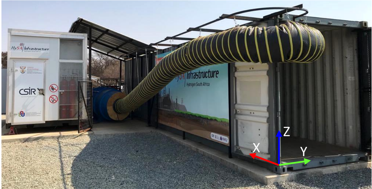
Figure 3-1: Experimental facility, showing the open boundary, including the fan and ventilation tube (HySA Mining Platform Test Facility for Green Mining).
