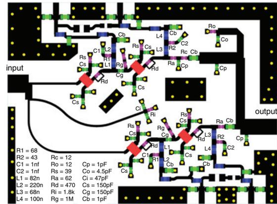
Fig. 1 PCB layout of amplifier
