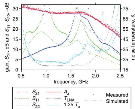
Fig. 2 Simulated and measured gain, input and output reflection coefficient and noise temperature
