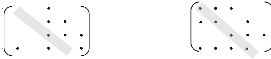
Figure 7.20: (a) Example of a \gamma block where \theta source symbols can be decoded (b) Example of a \gamma block where (\theta - 1) source symbols can be decoded
