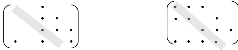
Figure 7.16: (a) Example of a \gamma block decodable without delay (b) Example of a \gamma block that is not decodable
