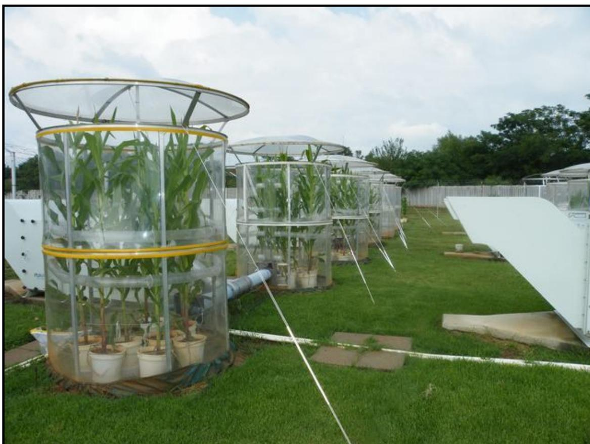
**Figure 3.2: Photo of the OTC facility at the Potchefstroom campus, North west University, during the December 2009/ January 2010 maize project, showing six of the twelve OTCs.**
