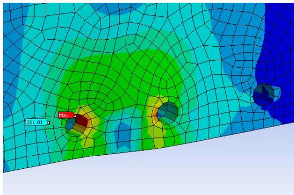
Figure 7.9: High stress gradient around hole joint.
