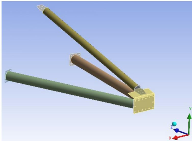
Figure 7.4: Finite element model of 3D cross arm.
