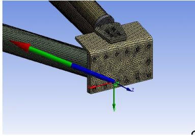
Figure 7.7: Reaction forces on revolute joint.
