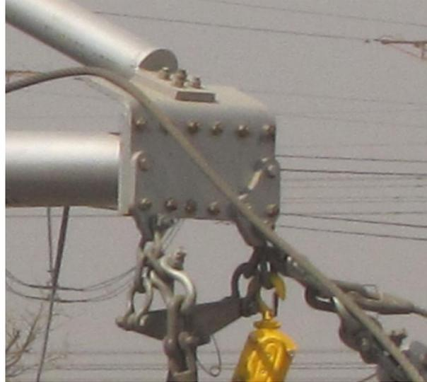
Figure 7.1: Photo showing the attachment of the load cells on the test structure cross arm.
