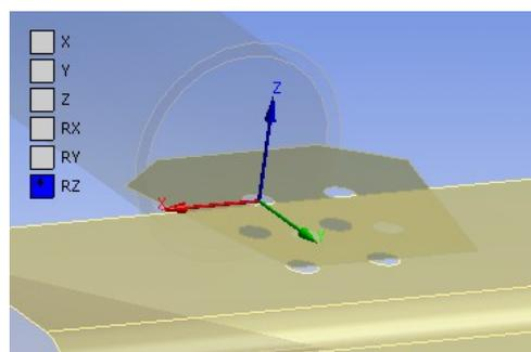
Figure 7.6: Revolute joint (Top 1A) indicating only rotation about the z-axis is permitted.
