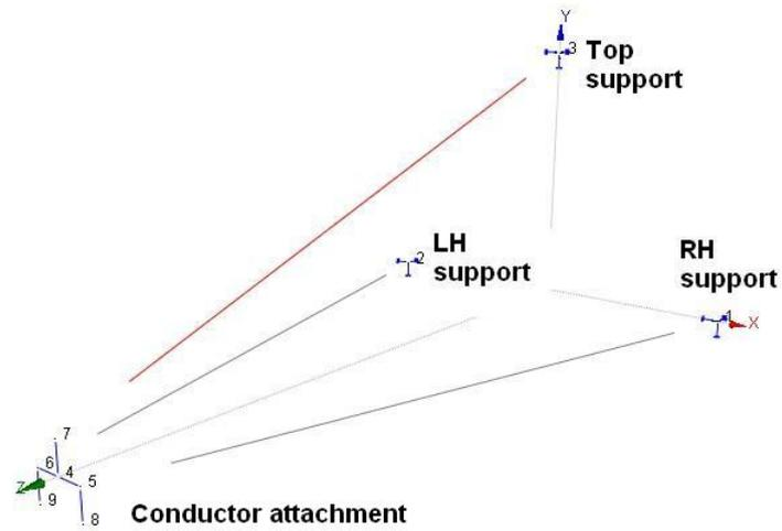
Figure 7.3: Prokon model 2: Improved cross arm model with specific end connection detail. The cross arm model consist of three main members that are fixed at the support and the conductor attachment end is more detailed with rigid links. Rigid represents only load transferring and not a structural member.
