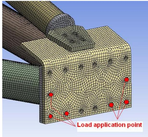
Figure 7.5: Cross arm mesh control display after mesh refinement.
