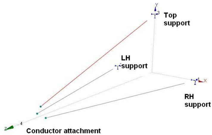
Figure 7.2: Prokon model 1: Tripod cross arm model - pinned. This cross arm has three main members that are fixed at the support and pinned at the conductor attachment end.
