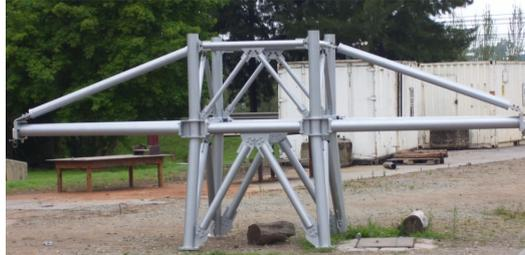
Figure 1.2: Picture showing the fabricated tubular test tower.
