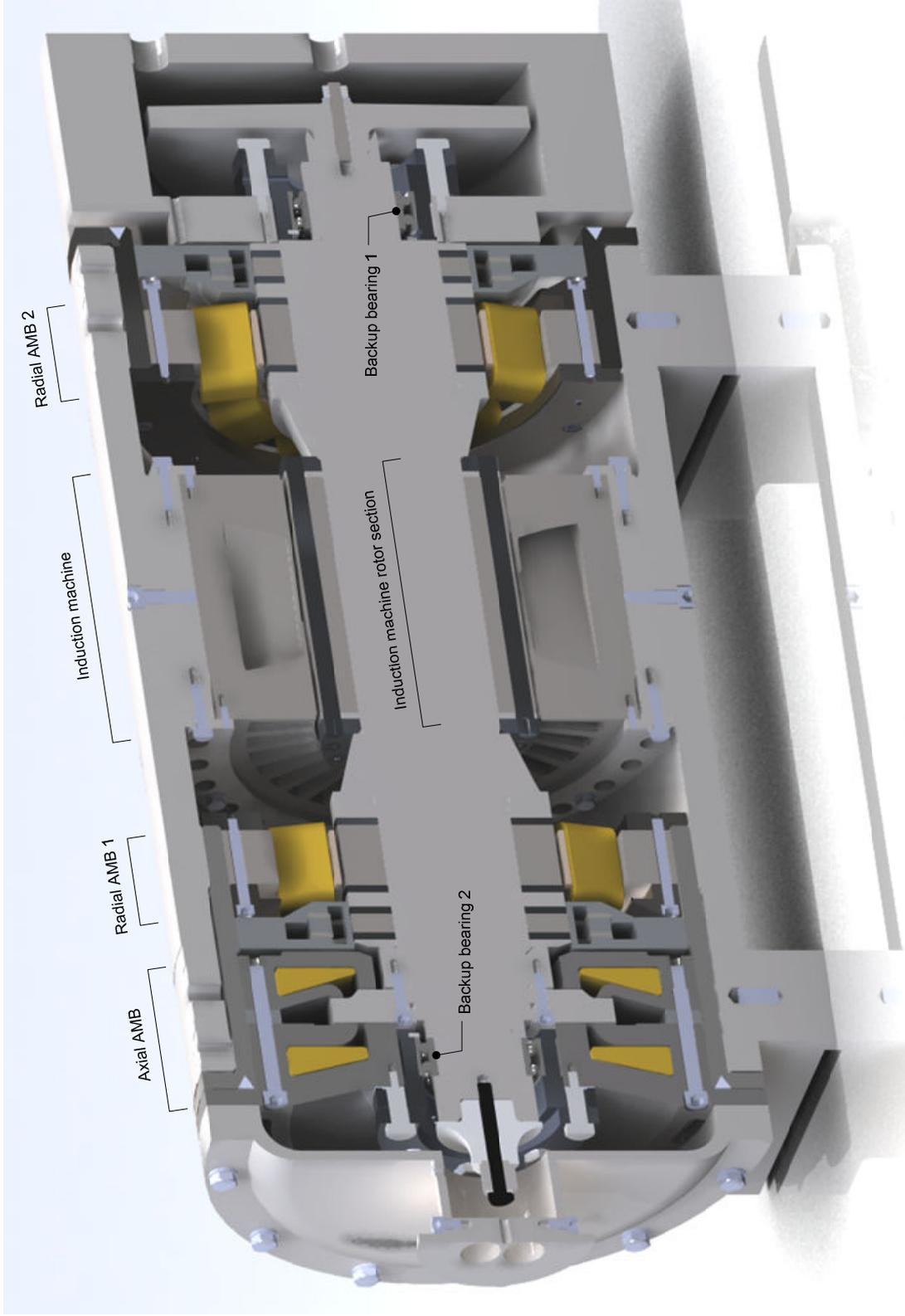
Figure 1-3: AMB supported high speed induction machine assembly
