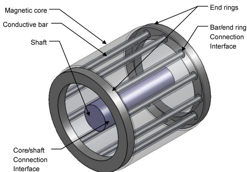
**Figure 1-2: Induction machine cage rotor illustration**
