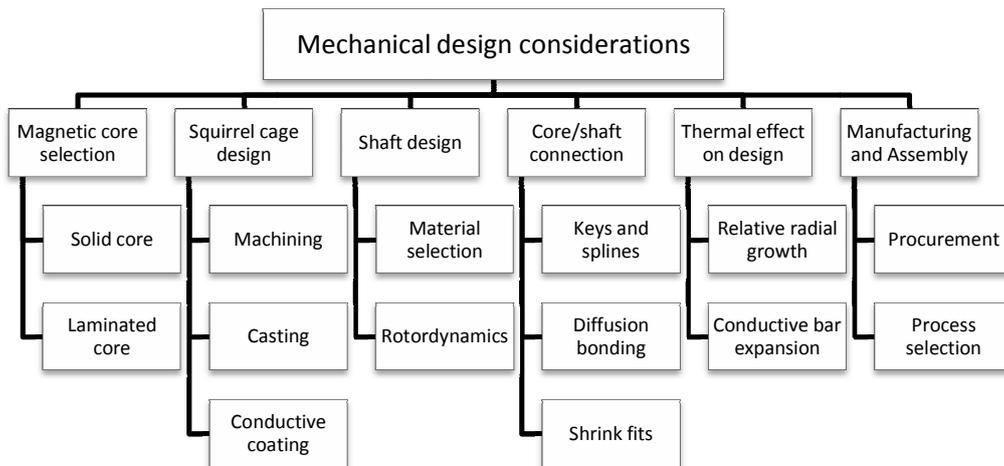
**Figure 1-4: Induction machine rotor's main design considerations**
