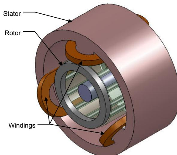
**Figure 1-1: Simple illustration of complete induction machine**
