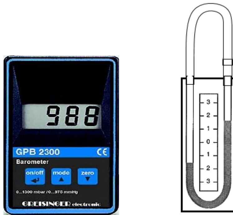
Figure 1-4: Barometer and vertical manometer (adapted from [24])
