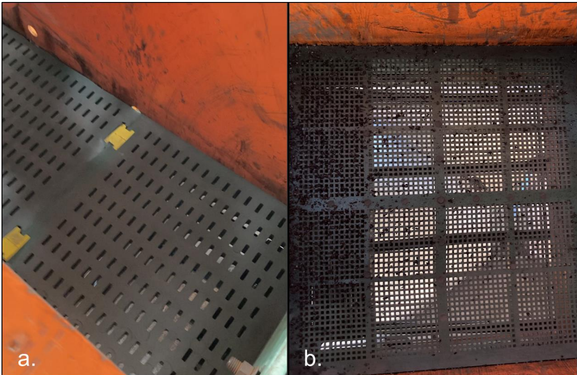
Figure 3.2: Photo of the panels used with a) the 5.6 mm panels and b) the 2.8 mm panels
