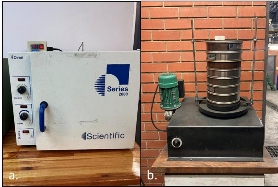
Figure 3.6: Photographs of a) the oven used and b) the sieve shaker used
