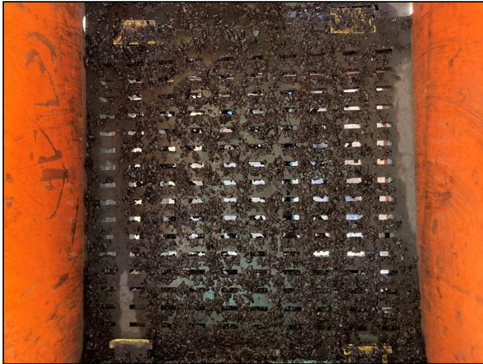
Figure 4.5: Photograph showing agglomeration of wet particles to the screen surface
