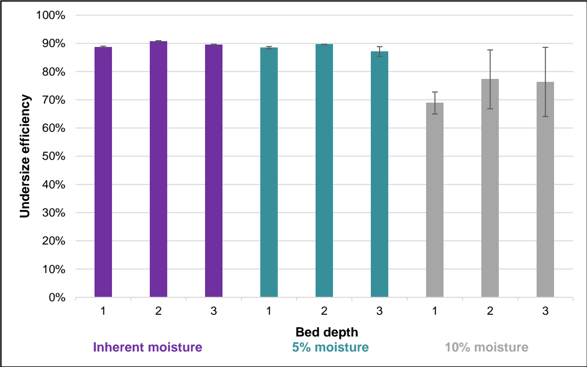
Figure 4.20: Undersize efficiencies with varying bed depths with the addition of a 0.5:1 ceramic to coal ratio
