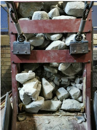
Figure 6-41: Partial unblocking for the first test at 50% excitation unbalance.
