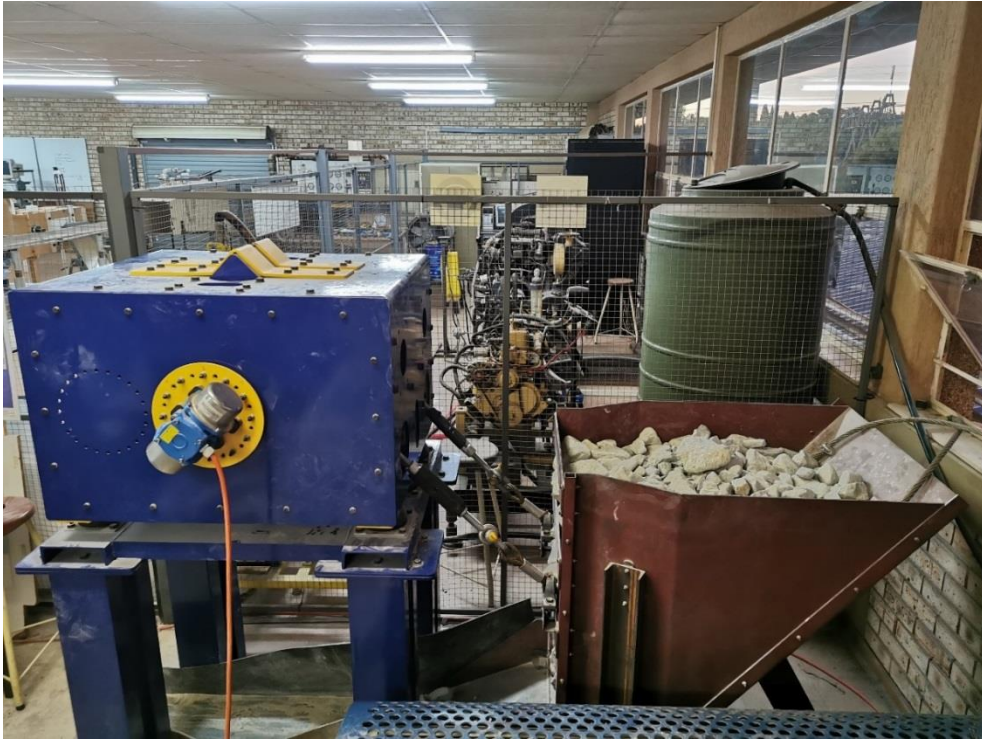
Figure 6-9: Machine with steel cables attached while caught in a blockage.
