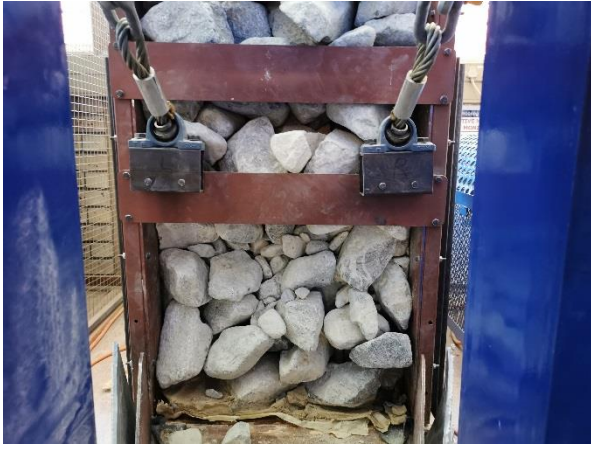
Figure 7-7: Blockage created for the second test where cables are caught in a cemented blockage.
