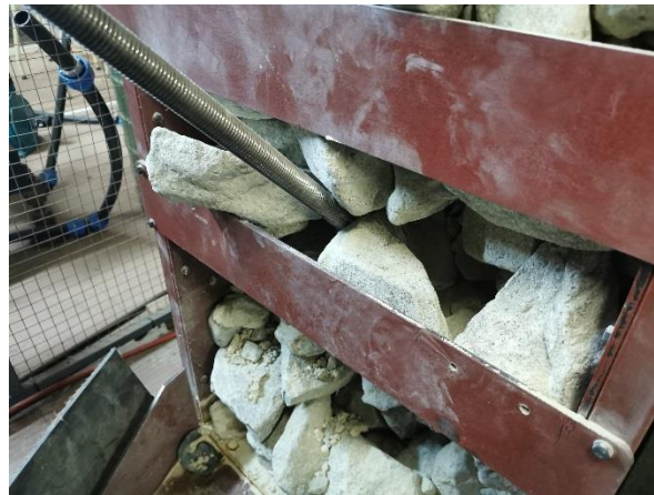
Figure 6-46: Representation of how the hammer made contact with the sample rock.
