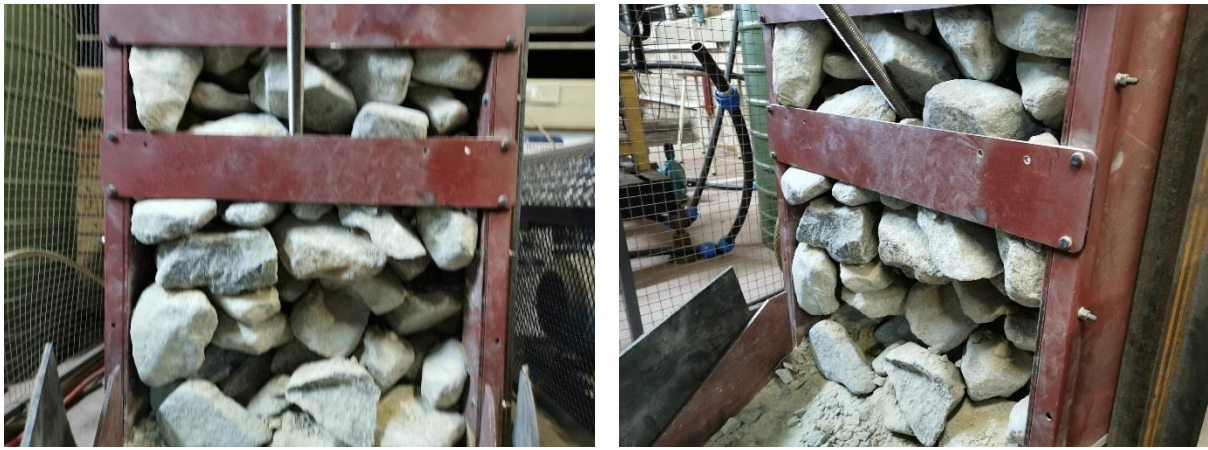
Figure 7-9: Blockage created for the second test where the hammer is for unblocking a dry interlocking blockage.
