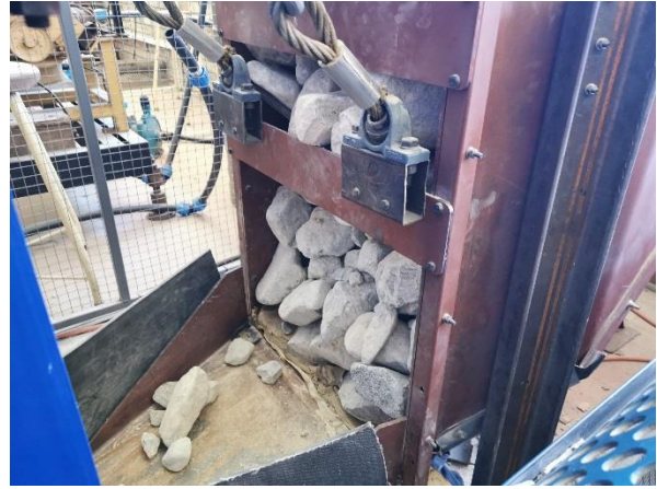
Figure 7-8: Partial unblocking for the second test, at 77 % excitation unbalance, where steel cables are used for unblocking a cemented blockage.
