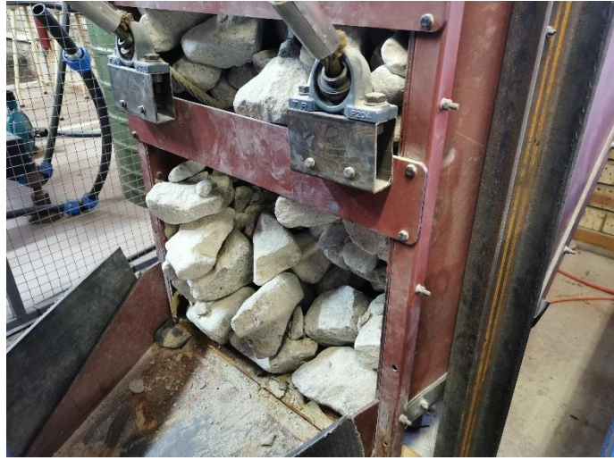
Figure 6-40: Blockage created for the first test where cables are caught in a cemented blockage.
