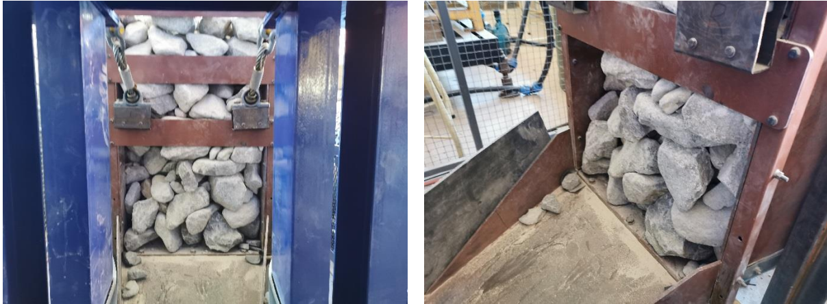
Figure 7-4: Blockage created for the third test frequency where steel cables are caught in a dry interlocking blockage.
