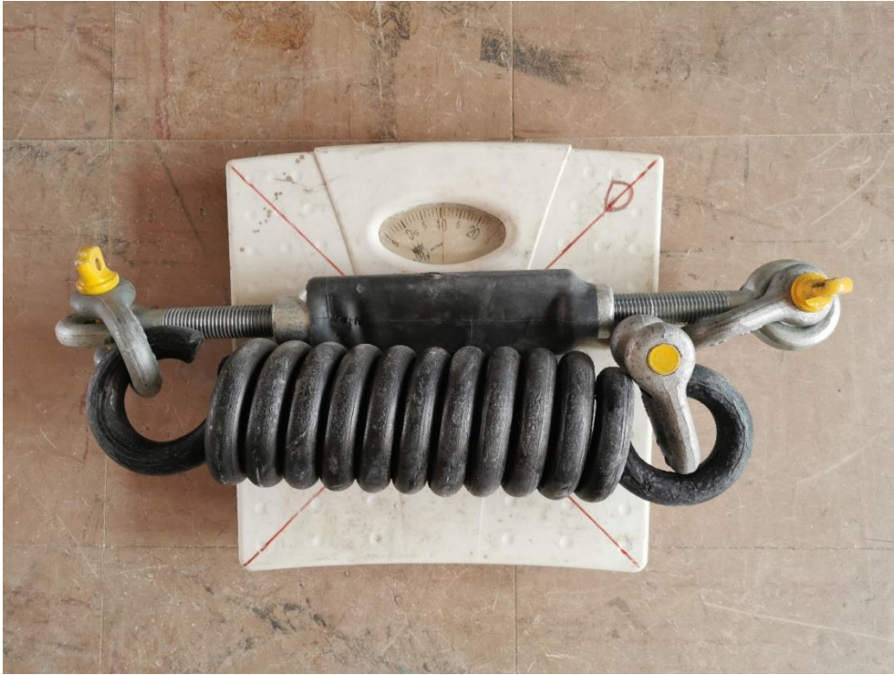
Figure 5-3: Representation of the turnbuckle, shackles and extension spring weighed by a household scale.
