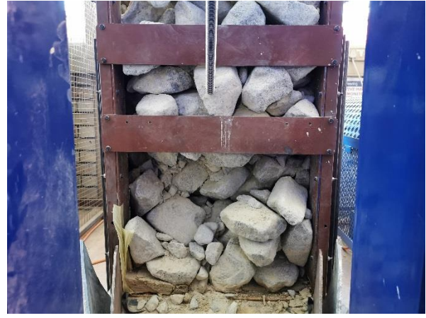
Figure 7-11: Blockage created for the second test where the hammer is used for unblocking a cemented blockage.
