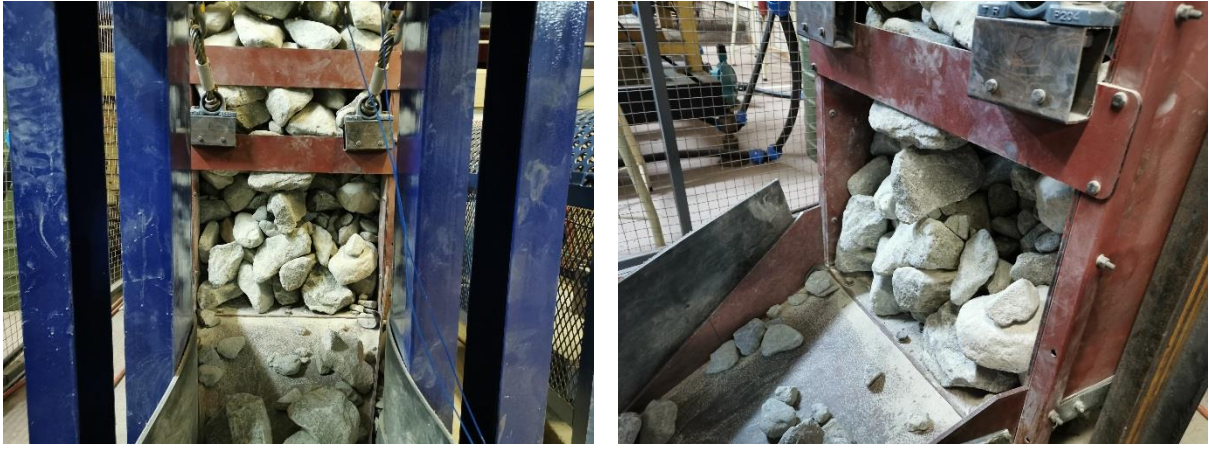
Figure 7-5: Partial unblocking occurred at 20.25 Hz and an unbalance of 94 % for the third test frequency where steel cables are used for unblocking a dry interlocking blockage.
