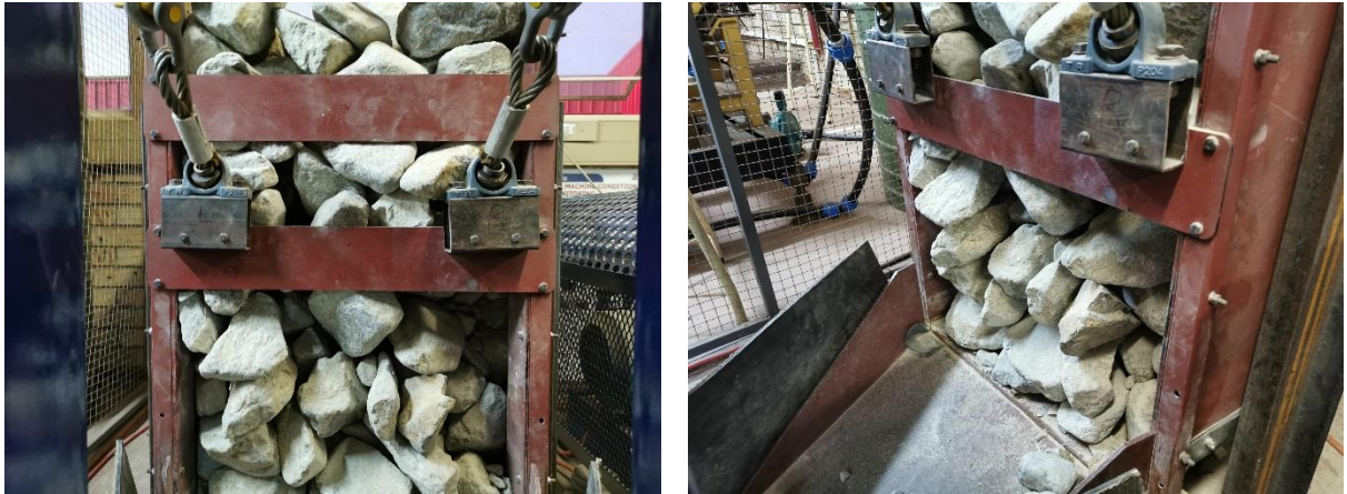
Figure 6-29: Blockage created for the first test frequency with the gate of the chute removed.
