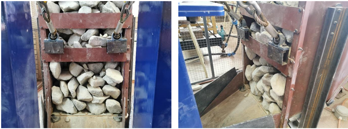
Figure 6-57: Blockage created for the constant load test where the steel cables are used for unblocking a dry interlocking blockage.
