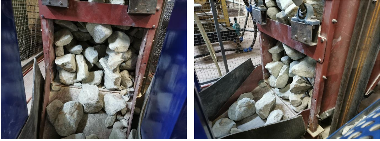
Figure 6-30: Partial unblocking occurred at 18.25 Hz and an unbalance of 77%.
