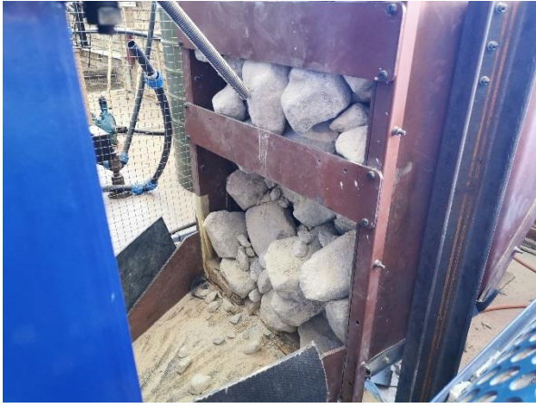
Figure 7-11: Blockage created for the second test where the hammer is used for unblocking a cemented blockage.
