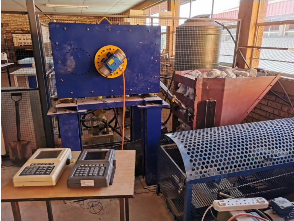
Figure 7-3: Representation of the test setup for the third test frequency where steel cables are caught in a dry interlocking blockage.
