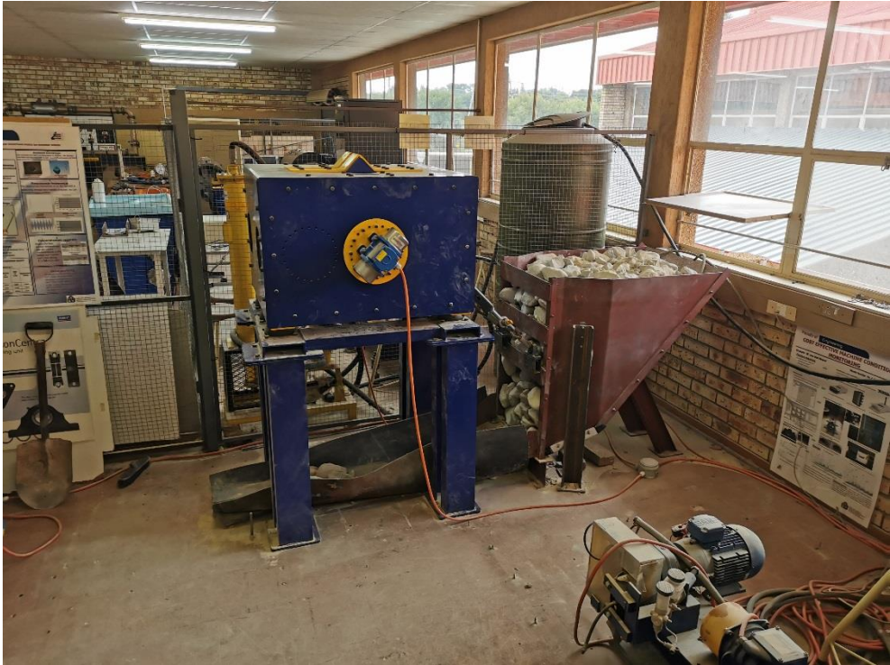
Figure 6-56: Representation of test setup for the constant load test where the steel cables are used for unblocking a dry interlocking blockage.
