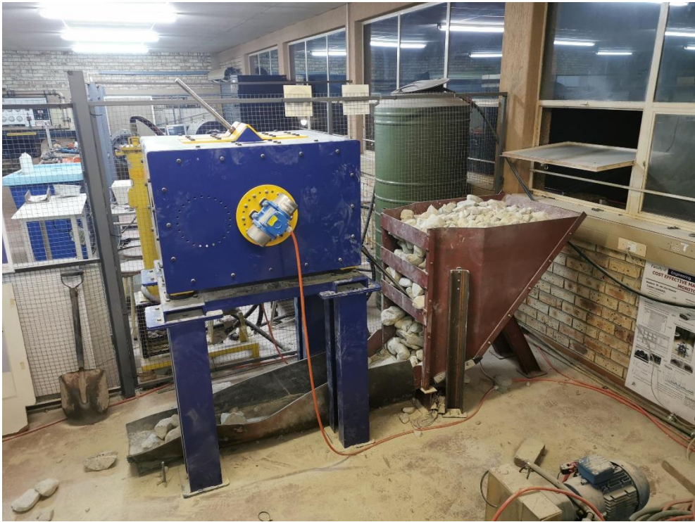
Figure 6-65: Representation of test setup for the fatigue based test where the hammer is used for unblocking a wet interlocking blockage.
