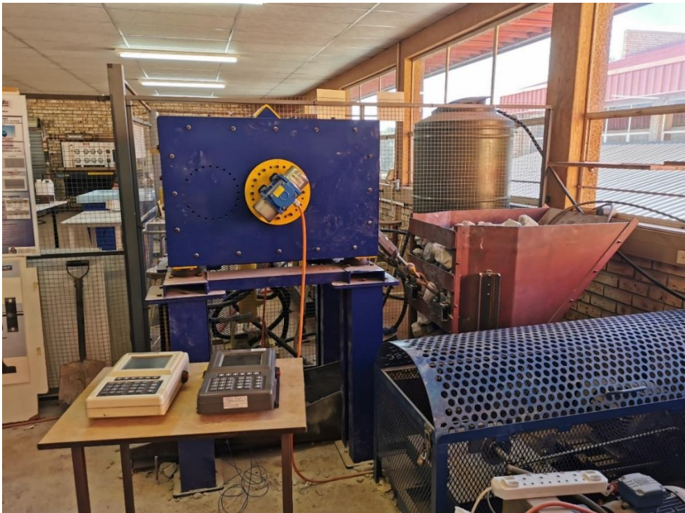
Figure 7-1: Representation of the test setup for the second test frequency where steel cables are caught in a dry interlocking blockage.
