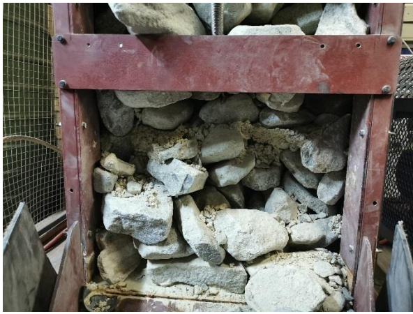
Figure 6-45: Blockage created for the first hammer test with the gate of the chute removed.
