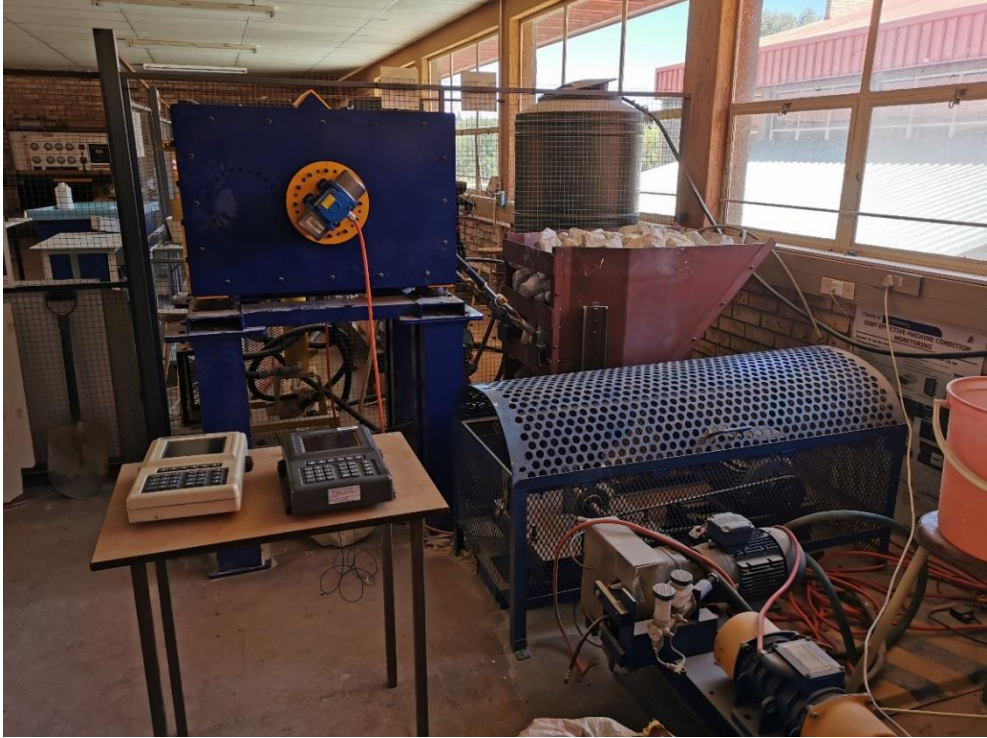
Figure 7-6: Representation of test setup for the second test where steel cables are caught in a cemented blockage.
