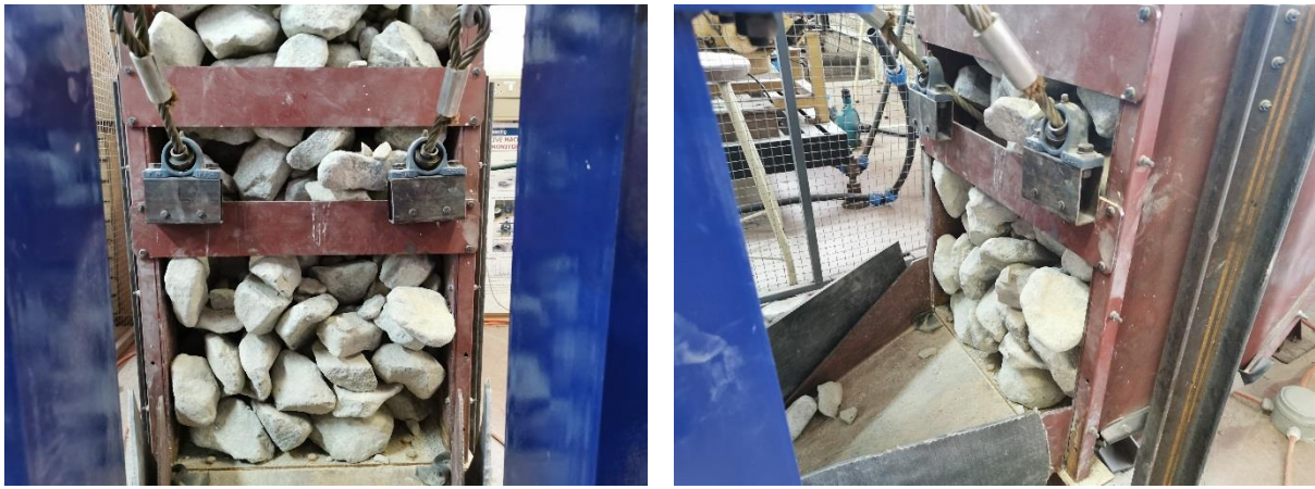
Figure 6-58: Representation of the blockage after 17 consecutive runs for the constant load method with steel cables.
