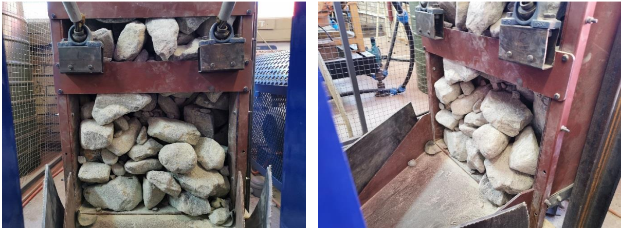
Figure 7-2: Blockage created for the second test frequency where steel cables are caught in a dry interlocking blockage.
