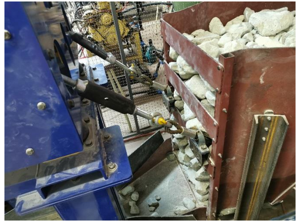
Figure 6-8: Representation of the steel cables attached to the machine. Left: Inside the machine. Right: Between the machine and scale chute.
