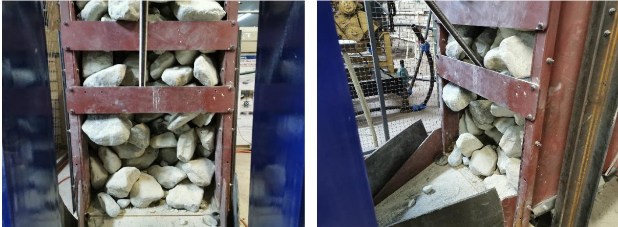
Figure 6-60: Blockage created for the constant load test where the hammer is used for unblocking a dry interlocking blockage.
