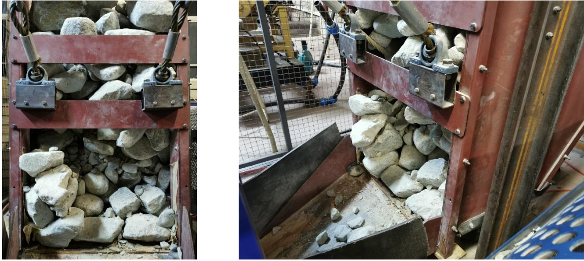
Figure 6-42: Partial unblocking for the first test at 64% excitation unbalance.
