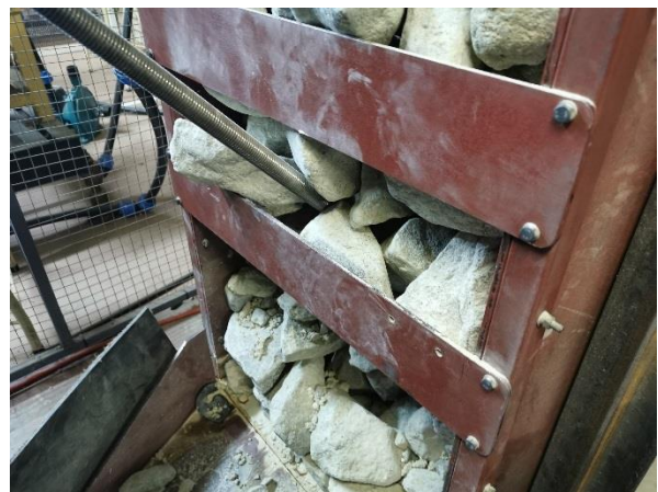
Figure 6-47: Representation of a small partial unblocking at an unbalance of 77%.
