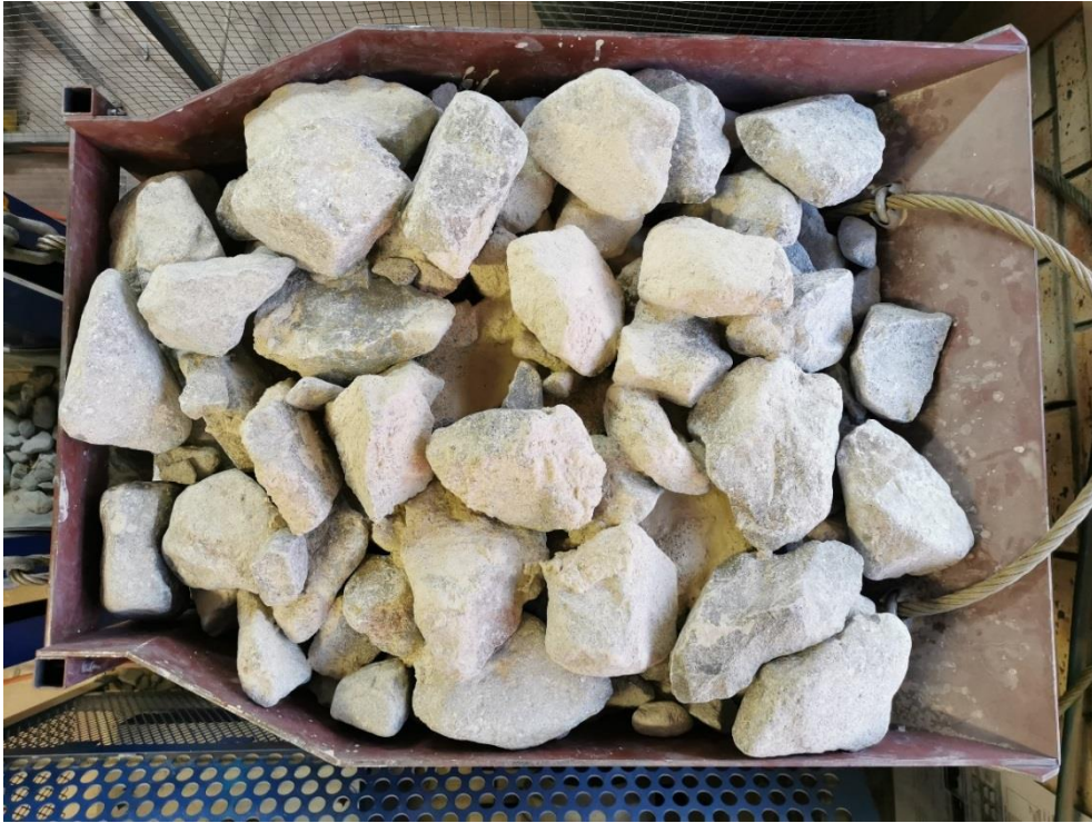
Figure 6-39: Top view of the scaled chute where mud was added and left to dry.
