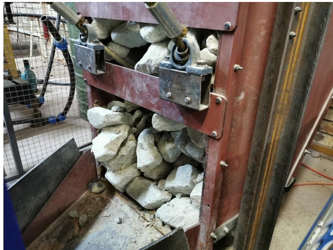
Figure 6-41: Partial unblocking for the first test at 50% excitation unbalance.
