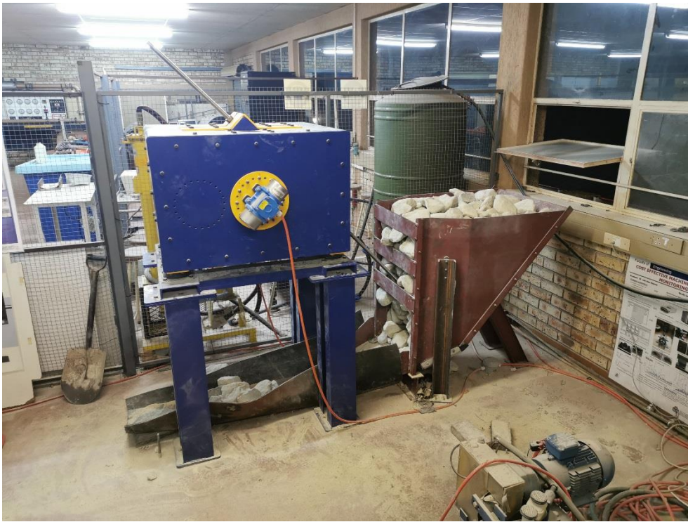
Figure 6-59: Representation of test setup for the constant load test where the hammer is used for unblocking a dry interlocking blockage.
