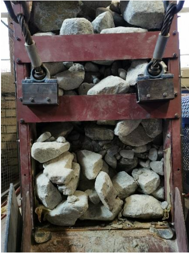
Figure 6-40: Blockage created for the first test where cables are caught in a cemented blockage.
