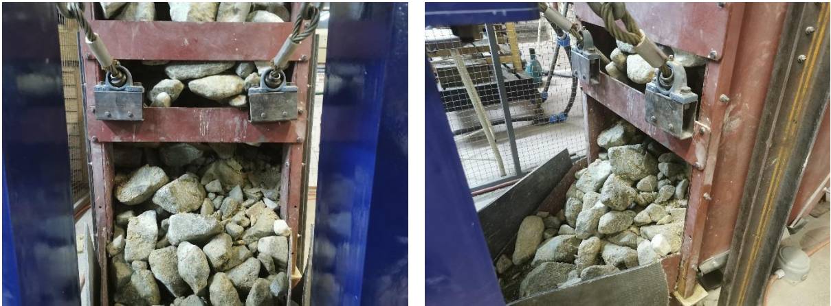
Figure 6-64: Representation of a successful unblocking of the wet interlocking blockage by using a constant load method with the steel cables.
