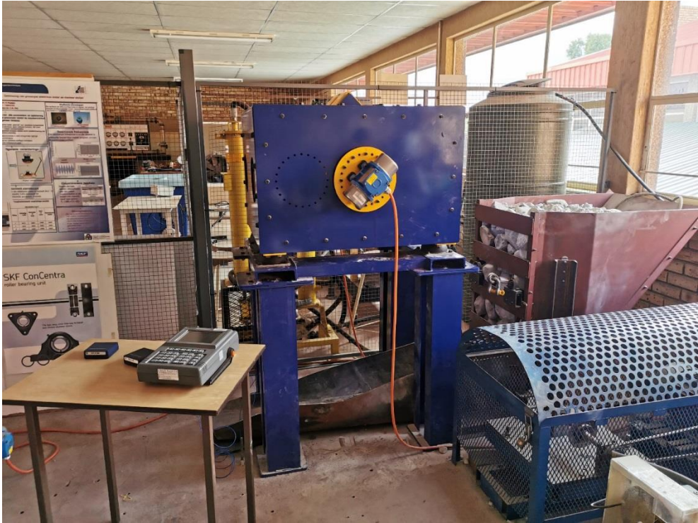
Figure 5-5: Stand-alone machine with Diagnostic Instrument coupled, with accelerometers.
