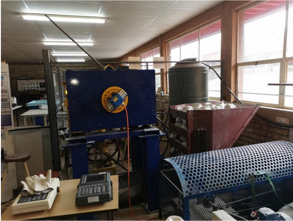
Figure 6-15: Machine with M24 threaded rod (hammer) attached.
