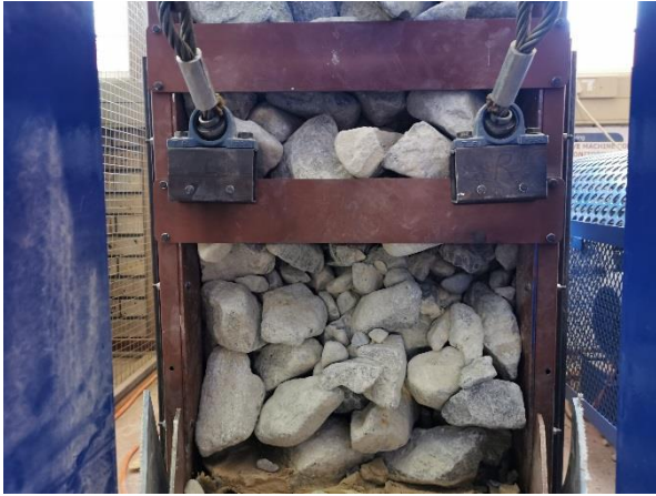
Figure 7-8: Partial unblocking for the second test, at 77 % excitation unbalance, where steel cables are used for unblocking a cemented blockage.
