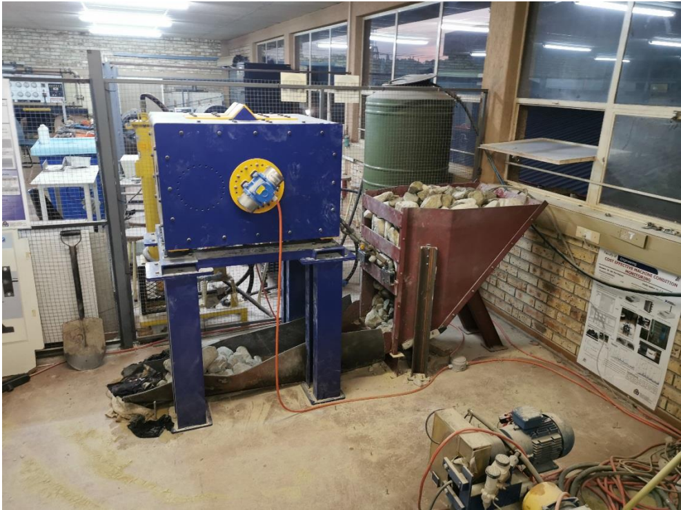
Figure 6-62: Representation of test setup for the constant load test where the steel cables are used for unblocking a wet interlocking blockage.
