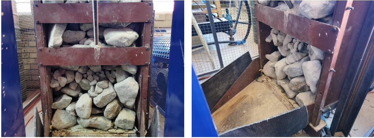
Figure 6-52: Blockage created for the first test where the hammer is used for unblocking a cemented blockage.
