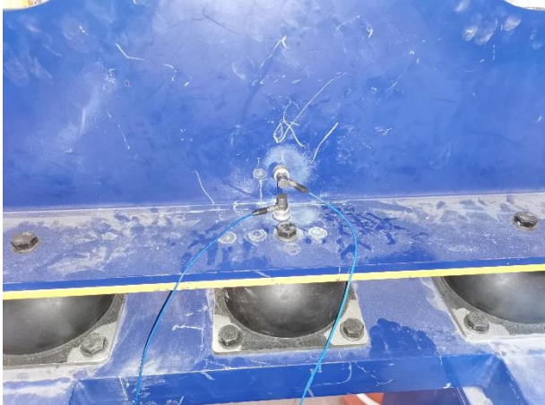
Figure 5-6: Placement of the accelerometer at the fixing point of the left rubber mounts.
