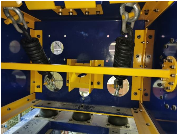
Figure 6-8: Representation of the steel cables attached to the machine. Left: Inside the machine. Right: Between the machine and scale chute.
