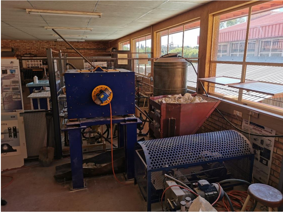
Figure 7-10: Representation of test setup for the second test where the hammer is used for unblocking a cemented blockage.
