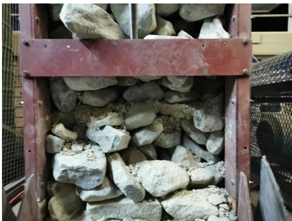
Figure 6-47: Representation of a small partial unblocking at an unbalance of 77%.
