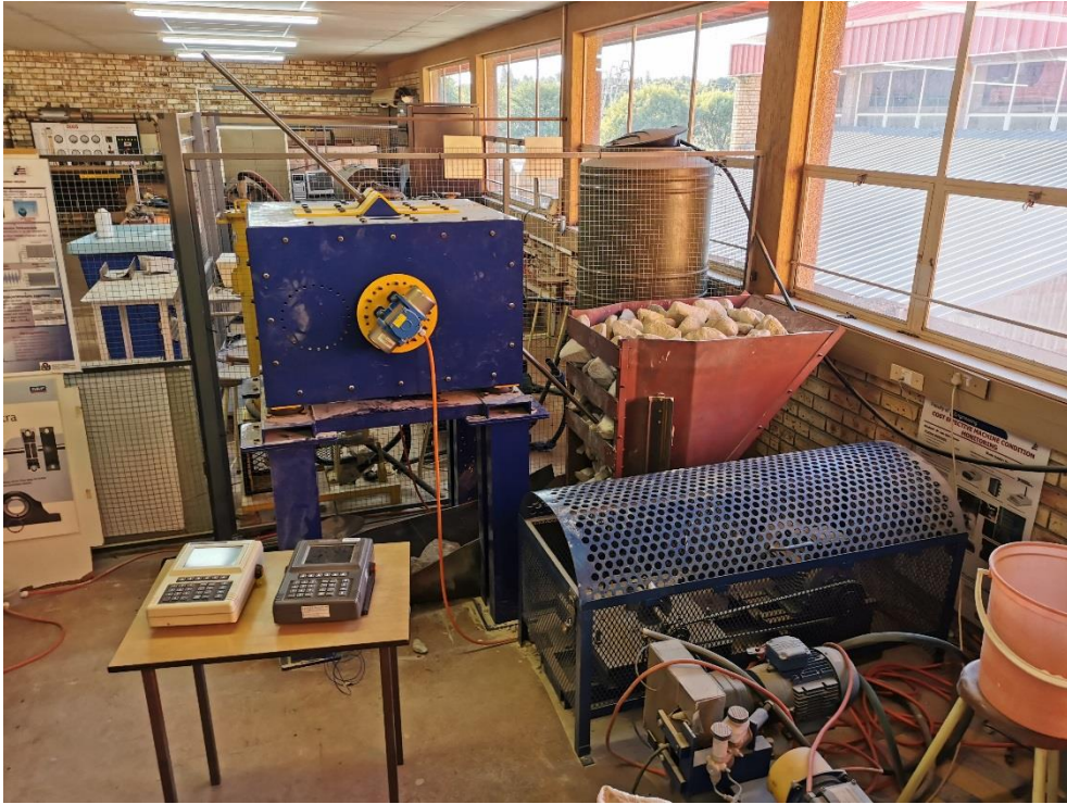
Figure 6-51: Representation of test setup for the first test where the hammer is used for unblocking a cemented blockage.
