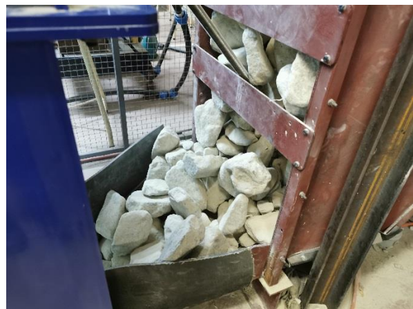
Figure 6-61: Representation of a successful unblocking of the blockage by utilizing a constant load method with the hammer operation.
