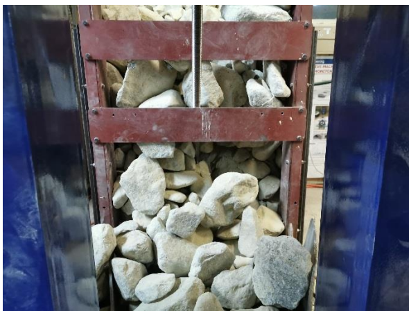
Figure 6-61: Representation of a successful unblocking of the blockage by utilizing a constant load method with the hammer operation.
