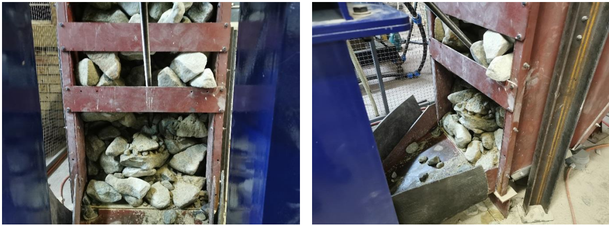
Figure 6-67: Representation of the blockage after 10 consecutive runs.
