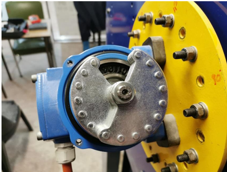
Figure 5-13: Close up of the discs forming the unbalance mass of the excitation motor.
