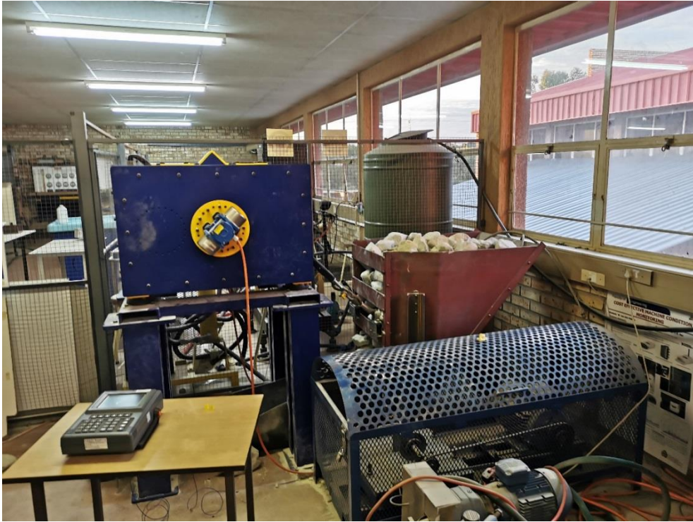
Figure 6-38: Representation of test setup for the first test where steel cables are caught in a cemented blockage.
