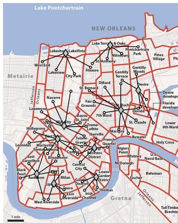
Figure 6.3 Set covering location model result indicating ten facilities
