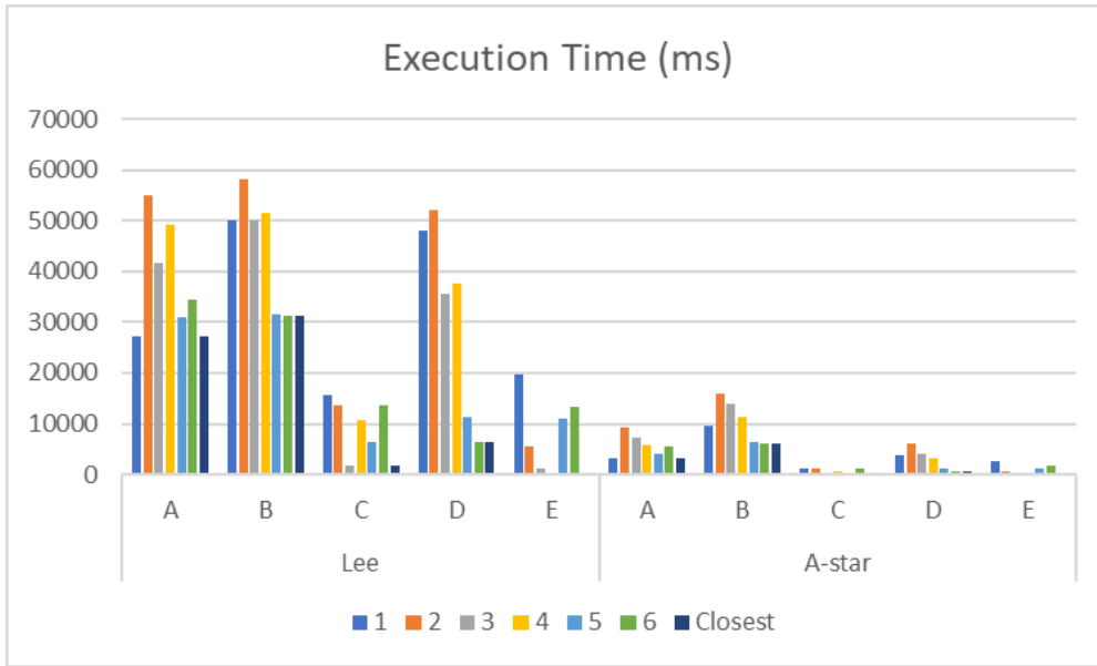
Figure 5.13 Graphical analysis of the execution time for the Lee and A-star algorithms
