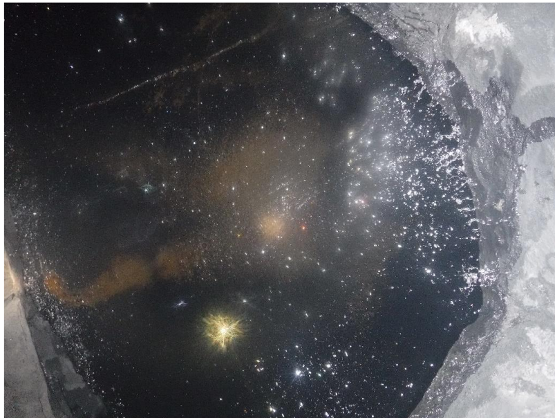
Figure I-4: Water plug identified in a raise borehole
