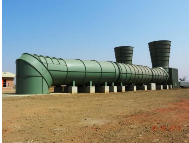
Figure 1-7: Surface extractor fan of a deep-level mine [12]
