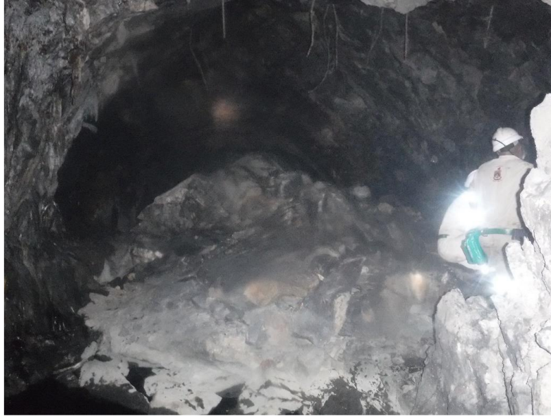
Figure I-3: Fall of ground in Zone 1 behind the main booster fans
