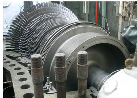
**Figure 7** – Steam Turbine Maintenance (Source; Sasol)
