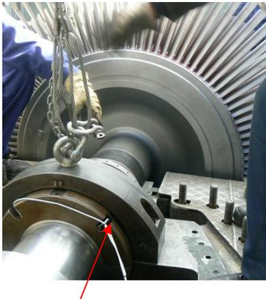
High vibrations signal received from probes on turbine
