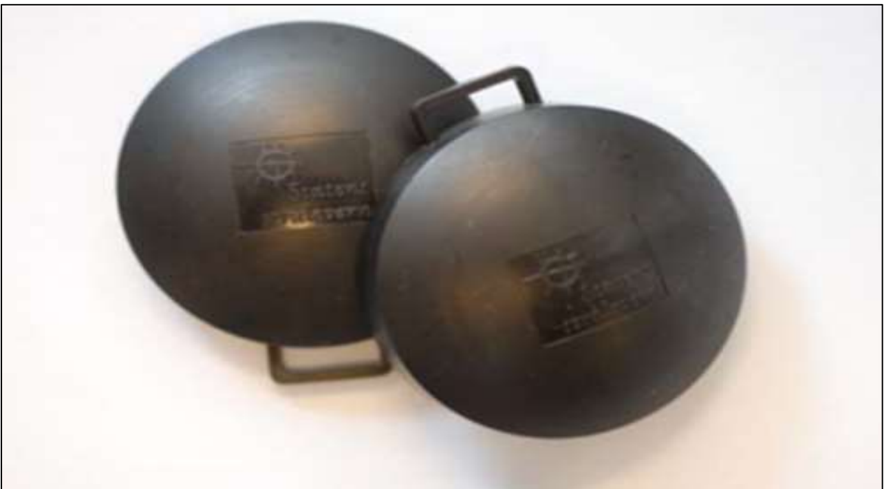
Figure 3.5: An illustration of CR-39 radon gas monitors
