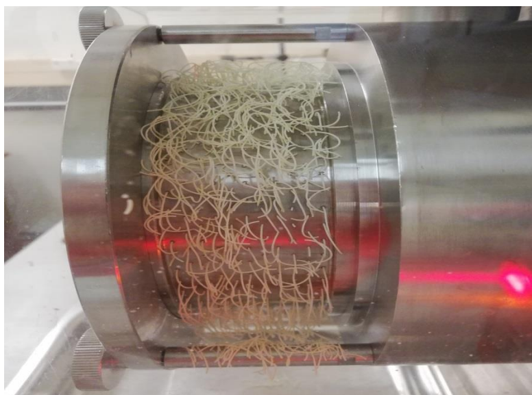
Figure E1: Side view of extruder pushing the wetted powder mass through the sieve
