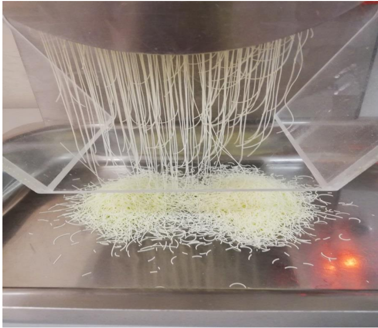
Figure E3: Front view of the extruder producing spaghetti like extrudate
